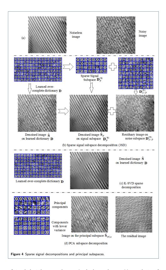
Let us look at the proposed sparse signal subspace decomposition on the top of Fig. 4(b) The 128 atoms  $\mathbf{d}_k$ s of the learned overcomplete dictionary  $\mathbf{D}$  are shown in descending order of their energies measured by  $\|\boldsymbol{\beta}_k\|_2$ . The 32 principal signal
