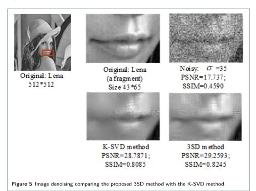
From the results shown in Fig. 5, the 3SD method outperforms the K-SVD method by about 1dB in PSNR and by about 1% in SSIM (depending on how much details in images and how faint the details). In terms of subjective visual quality, we can see that the corner of mouth and the nasolabial fold with weak intensities are much better recovered by 3SD method.
