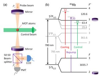
FIG. 1. (a) Schematic of the experimental setup. (b) Energy levels diagram of <sup>85</sup>Rb. The black (grey) lines represent energy levels relevant (not relevant) for the present experiment. The frequency spacing between consecutive *F* levels and the detuning of the lasers are marked (in MHz).
