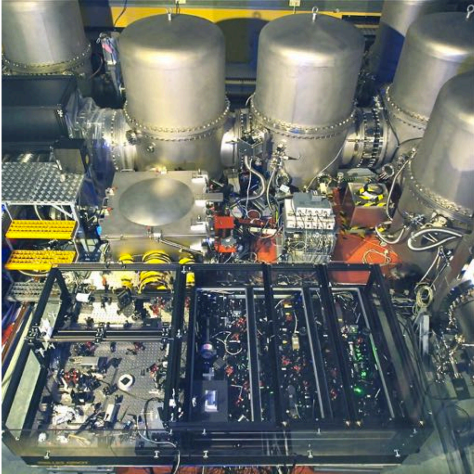
Figure 30: GEO 600 – View into the central building of the British-German GW detector located close to Hannover, Germany. The vacuum chambers contain the suspended beam splitter, power- and signal recycling mirrors, additional input and output optics as well as mirrors to realize a double pass of the laser light through the 600 m long interferometer arms. By courtesy of the AEI.
