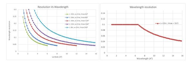
Figure 3: (a) Wavelength resolution for various instrument lengths and a neutron pulse length of 2 ms. For a repetition rate of 20Hz, the longer the instrument, the shorter the frame overlap wavelength. (b) Wavelength resolution which can be achieved on a 12 m instrument with a double disk chopper.
