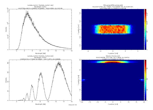
Figure 4: McStas simulation of a 12m neutron reflectometer with a 10x5 cm<sup>2</sup> sample (Ni 20nm//Si) at an incidence angle of 3°. (a) Wavelength distribution incident on the sample. (b) Incident neutron distribution on the sample. (c) Wavelength spectrum measured in the specular reflectivity direction. (d) Neutron intensity on a PSD at 2 m from the sample. The top horizontal line corresponds to the reflected signal on the PSD detector
