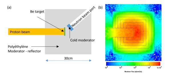
Figure 1: (a) Sketch of a compact Target and moderator assembly. The target is a sheet of beryllium of thickness ~1mm and of surface 25-100cm<sup>2</sup>. The moderator is a hydrogenated material (PE) which allows keeping short thermal neutron pulses. The assembly is surrounded by polyethylene, graphite or beryllium acting as reflectors. (b) Thermal neutron flux of such a source (without the cold moderator).
