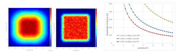
Figure 2: (a) Illumination of the sample for an L/D = 80 radiography instrument. The flux in the central  $20x20cm^2$  part is on the order of  $2x10^7$  n/s/cm<sup>2</sup>. (b) Illumination of the sample for an L/D = 240 radiography instrument. The flux in the central  $40x40cm^2$  part is very homogeneous but reduced to  $2x10^6$  n/s/cm<sup>2</sup>. (c) Wavelength resolution for various instrument lengths at  $w = 400\mu s$  and f = 25Hz.
