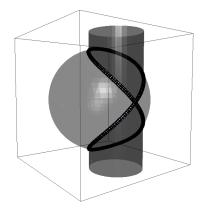
Figure 2: Viviani's curve as the intersection of a sphere with a cylinder.
