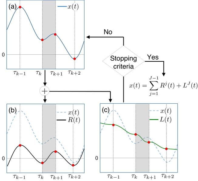
Fig. 2: Flow chart showing the recursive decomposition of (a) signal  $x(t)$  into (b) a rotation component  $R(t)$  and (c) a baseline component  $L(t)$ . The highlighted region shows the support of the intrinsic basis function defined between two consecutive extrema,  $\tau_k$  and  $\tau_{k+1}$ .
