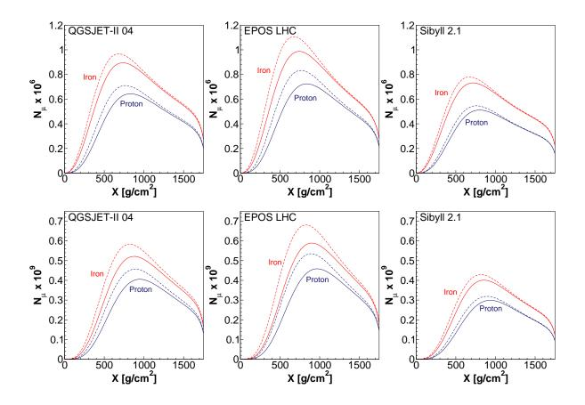
FIG. 10: Predictions for the average longitudinal profiles of muons for air showers generated by protons and iron nuclei with primary energies of  $10^{17}$  eV (upper panels) and  $10^{20}$  eV (lower panels). Solid (dashed) lines represent the full (non - diffractive) simulations.
