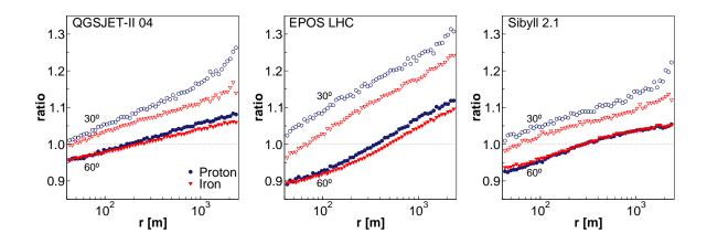
FIG. 11: Ratio between the predictions for muon densities obtained considering only non - diffractive interactions and those derived including diffractive and non - diffractive interactions as a function of the distance to the shower core. Showers initiated by protons (iron nuclei) are represented by blue circles (red triangles). Solid (open) symbols denote showers initiated by primary reaching the atmosphere with a zenithal angle of  $60^{\circ}$  ( $30^{\circ}$ ).
