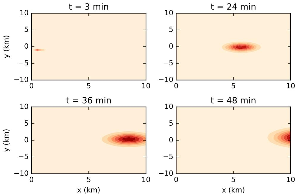
Figure 1: **The dynamics of one puff.** This figure shows the concentration surface of one puff at different time. The release occurs at  $t = 0$  and the release location is  $(0, -1163.5 \text{ km})$ . The wind direction is  $0.17 \text{ m/s}$  and the wind speed is  $4 \text{ m/s}$ .  $p_y$  and  $q_y$  are  $0.466$  and  $0.866$  respectively. Note the color bar is different for each plot.
