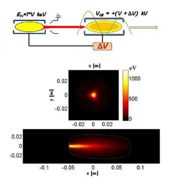
Fig. 13. Scheme of the Charge Breeding Technique: a radioactive beam is extracted from a hot  $1^+$  source, and injected into the charge breeder to enhance its charge state (top figure). Spatial distribution of the energy released by the injected particles inside the plasma on the xy plane and xz plane (central and bottom figures).
