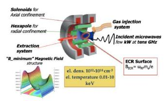
Fig. 1. Sketch of the experimental setup of a B-minimum magnetic trap, with typical values of density and temperature achievable in last-generation machines.
