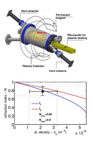
Fig. 9. First measurement of plasma density in a compact plasma trap (bottom) and the relative experimental setup implemented at INFN-LNS for the installation of the VESPRI interferometer (top) [57,58].
