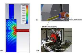
Fig. 6. Quasi-optical RF launching setup installed in the Flexible Plasma Trap (FPT): a) simulation of the Electromagnetic Wave in-trap injection; b) mechanical drawing of the wave guides inside the PST; c) photo of the FPT showing the launcher [52]
