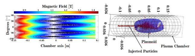
Fig. 16. Left side: distribution of ion losses on the plasma chamber wall. Right side: distribution of the particles captured by the plasma[65].
