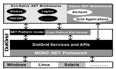
Figure 2 Current developed DotGrid services and APIs
