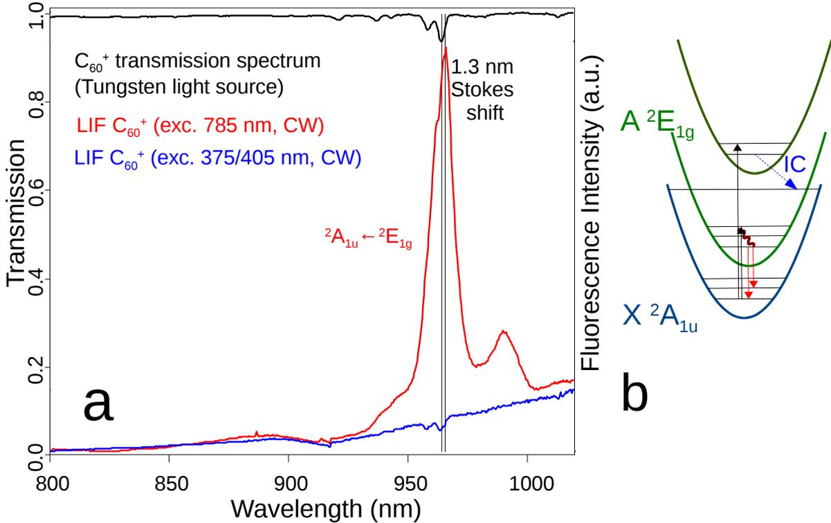
FIG. 1: (a) Spectroscopic measurements on  $C_{60}^+$  containing cryogenic neon matrixes as indicated. (b) Energy level diagram rationalizing these observations in terms of radiative (red arrows) and non-radiative decays.
