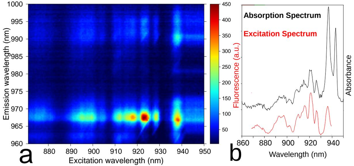
FIG. 2: **(a)** Fluorescence excitation/emission map obtained by tunable pulsed laser irradiation of a  $C_{60}^+$  containing neon matrix. **(b)** Fluorescence excitation spectrum (integrated emission as a function of excitation wavelength) in comparison to the absorption spectrum of  $C_{60}^+$ .
