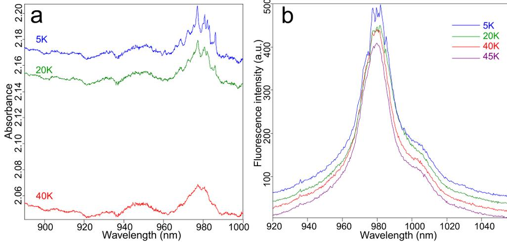
FIG. 6: **(a)** Absorption spectra of  $C_{60}^{+/-/0}$  in Kr matrix at various temperatures. The offset is real and is caused by changes of the optical properties of solid krypton, which lead to increased light scattering as the sample is cooled below 40 K. **(b)** LIF spectra of  $C_{60}^{+/-/0}$  in Kr matrix at various temperatures (785 nm excitation). Original spectra have a similar baseline. A vertical offset was added to better distinguish the individual spectra.
