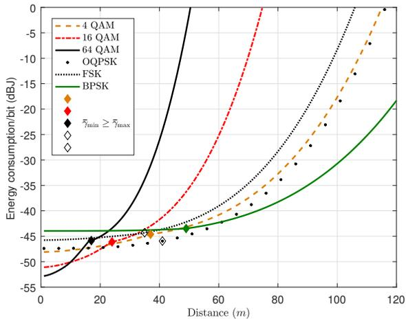
Fig. 3. Energy consumption of the modulation schemes with optimal required SNR at each distance. The marked condition  $\bar{\gamma}_{\min} \geq \bar{\gamma}_{\max}$  shows the distance beyond which the reliability constraints are not satisfied. Simulation parameters:  $P_0 = 10\text{mW}$ ,  $\varepsilon = 0.001$ ,  $\tau_r^{\max} = 3$ ,  $n_p = 984$ ,  $n_h = 40$ .
