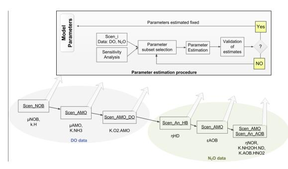
Figure 1 – Schematic of the parameter estimation procedure.
