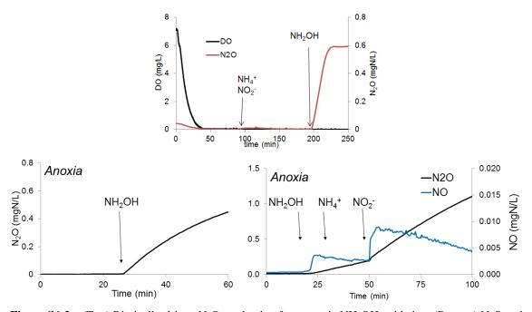
Figure S6-2 – (Top) Biotically-driven N<sub>2</sub>O production from anoxic NH<sub>2</sub>OH oxidation. (Bottom) N<sub>2</sub>O and NO liquid concentrations from anoxic NH<sub>2</sub>OH oxidation (left, NO<sub>2</sub><sup>-</sup> < 0.05 mgN/L at the end of the experiment), and anoxic NH<sub>2</sub>OH oxidation followed by NH<sub>4</sub><sup>+</sup> and NO<sub>2</sub><sup>-</sup> addition (right).
