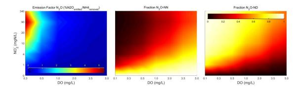
Figure 6 – Scenario analysis using the validated NHDA simulation model. Simulations were run under constant DO levels (0.1 - 0.3 - 0.5 - 1.0 - 2.0 - 3.5 - 5.0 mg/L), NO<sub>2</sub><sup>-</sup> (0 - 1 - 4 - 10 - 20 - 90 - 340 mgN/L). (Left) N<sub>2</sub>O emission factor (% N<sub>2</sub>O/NH<sub>4</sub><sup>+</sup>), colorbar: 0 - 5%, blue - red. (Middle, Right) NN, ND Pathway contribution ( - ), colorbar: 0 - 1, black - white.
