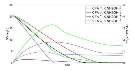
**Figure S4-2** – DO model simulation for an  $NH_4^+$  pulse ( $\mu_{MAX,AMO} = \mu_{MAX,HAO}$ ,  $K_{O2,AMO} = K_{O2,HAO}$ , pH = 7.5, 25 °C) to study the effect of NH<sub>3</sub> and NH<sub>2</sub>OH affinities to the DO and NH<sub>2</sub>OH concentration profiles. DO (straight lines), NH<sub>2</sub>OH (dotted line). ( $K_{FA=NH3} = 0.01 - 0.1 \text{ mgN/L}$ ,  $K_{NH2OH} = 0.2 - 2.4 \text{ mgN/L}$ ).
