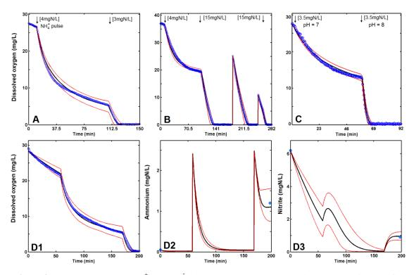
**Figure 4** – Experimental DO, NH<sub>4</sub><sup>+</sup> and NO<sub>2</sub><sup>-</sup> (blue markers) and model predictions (black line best-fit, red lines 95% CI). Datasets from Scen\_AMO, calibration: A and B; validation: C and D.
