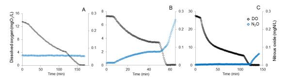
**Figure 2** – Dissolved oxygen and liquid nitrous oxide concentrations during experiments: Scen\_NOB  $(NO_2^- pulses)$  (A), Scen\_HAO (NH<sub>2</sub>OH pulses) (B) and Scen\_AMO (NH<sub>4</sub><sup>+</sup> pulses) (C) (3-4.5 mgN/L).
