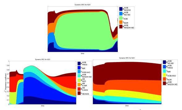
**Figure S2-2** – Dynamic sensitivity analysis for N<sub>2</sub>O: (Top) Scen\_AMO (NH<sub>4</sub><sup>+</sup> pulses). (Bottom) Scen\_An\_AOB (left: NH<sub>2</sub>OH followed by NO<sub>2</sub><sup>-</sup> pulse; right: NH<sub>2</sub>OH pulse). Only parameters with squared beta ( $\beta^2$ ) larger than 0.02 at some point of the batch are shown.
