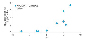
Figure S6-4 - Abiotic N<sub>2</sub>O production rates for NH<sub>2</sub>OH pulses (1.2 mgN/L) at varying pH.
