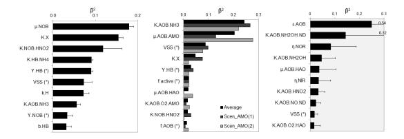
Figure 3 – Parameter sensitivity ranking of scenarios used during calibration for DO (white background) and N<sub>2</sub>O (grey background). Scen\_NOB (left), Scen\_AMO (middle and right). (\*) Parameters not considered for calibration.
