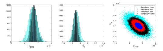
Figure S5-3. Samples from  $\mu_{NOB}$  and  $k_H$  estimates for different data frequencies used for calibration (every 0.5-2-5-10 minutes).
