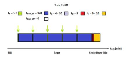
**Figure S1-1** – Operation regime for the parent nitritating SBR: 5 feeds / cycle (green), aerated during 320 minutes (blue), settling (pink), decanting (red) and idle phase (yellow).
