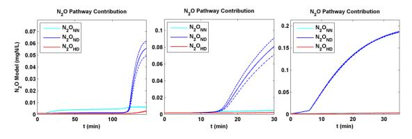
Figure S7-1 – Pathway contribution to the total N<sub>2</sub>O pool and 95%CI from calibrated parameters for: (Left, Middle) Scen\_AMO (NH<sub>4</sub><sup>+</sup> pulses, Aerobic  $\rightarrow$  anoxic), (Right) Scen\_HAO (NH<sub>2</sub>OH pulse, anoxic).
