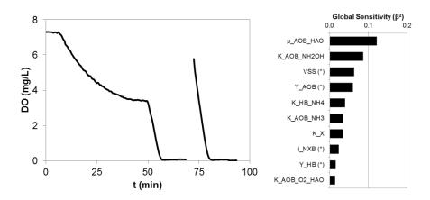
Figure S4-3 - Left: DO measurements during NH<sub>2</sub>OH oxidation at varying NH<sub>2</sub>OH levels (1.6mgN/L t = 7 min, 4 mgN/L t = 50 min, 4 mgN/L t = 52 min, 4 mgN/L at t = 75 min). Right: Corresponding DO-associated sensitivity ranking.
