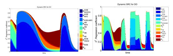
**Figure S2-1** – Dynamic sensitivity analysis for DO: Scen\_AMO (NH<sub>4</sub><sup>+</sup> pulses). Only parameters with squared beta ( $\beta^2$ ) larger than 0.02 at some point of the batch are shown.
