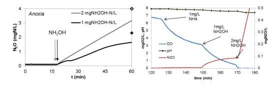
**Figure S6-3** – (Left) N<sub>2</sub>O concentration after anoxic NH<sub>2</sub>OH spikes under excess NO<sub>2</sub><sup>-</sup> (Markers, final N<sub>2</sub>O concentrations). (Rigth) DO, pH and N<sub>2</sub>O profiles after aerobic NH<sub>4</sub><sup>+</sup> (1mgN/L), NH<sub>2</sub>OH (1 and 2 mgN/L) spikes (Scen\_HAO).
