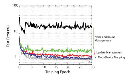
**Figure 6.** Test error of CNN with the MNIST dataset. Open white circles correspond to the model with the training performed using the floating point numbers. Lines with different colors correspond to RPU-baseline model with different management techniques enabled progressively.
