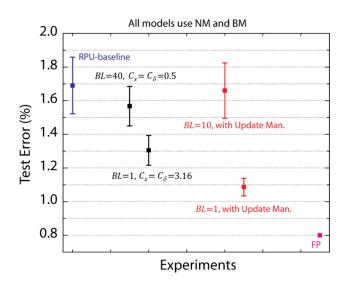
**Figure 5.** Average test error achieved between 25<sup>th</sup> and 30<sup>th</sup> epochs for a various RPU models with varying update schemes. Black data points correspond to updates with amplification factors that are equally distributed to the columns and the rows. Red data points corresponds to models that uses the update management scheme. RPU-baseline with noise and bound management as well as the FP-baseline models are also included for comparison.
