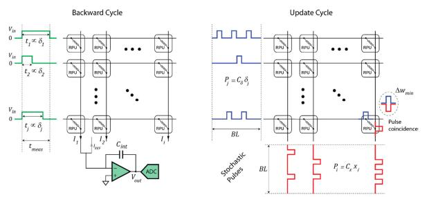
**Figure 2.** Schematics of an RPU array operation during the backward and update cycles. The forward cycle operations are identical to the backward cycle operations except the inputs are supplied from the columns and the outputs are read from the rows.
