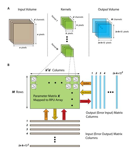
**Figure 1.** (**A**) Schematics of a convolutional layer showing the input volume, kernels, and the output volume. (**B**) Schematics of a mapped convolutional layer to an RPU array showing the input and output matrixes and their propagation through the kernel matrix during the forward, backward and the update cycles.
