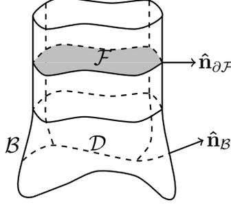
FIGURE 1. An illustration of the domain  $\mathcal{D}$  with boundary  $\partial\mathcal{D} = \bar{\mathcal{F}} \cup \mathcal{B}$  for the linearized problem in (3). We assume  $\hat{\mathbf{n}}_{\partial\mathcal{F}}$  agrees with  $\hat{\mathbf{n}}_{\mathcal{B}}$  on  $\partial\mathcal{F}$ .
