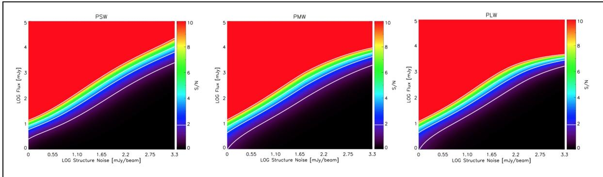
Figure 1.18: Log-log contour plot of the SNR values as a function of structure noise and source flux for the PSW, PMW and PLW arrays (left to right). SNR levels of 1, 3, 5 and 10 are overplotted with white contour lines.
