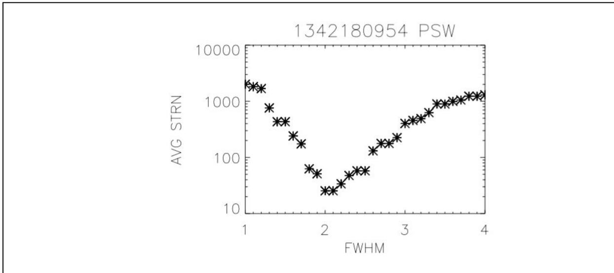
Figure 1.15.: The average structure noise value around the injected sources of 20 Jy into a 250 $\mu$ m map, as a function of the angular separation between the target pixel and the annulus, in units of the beam FWHM.
