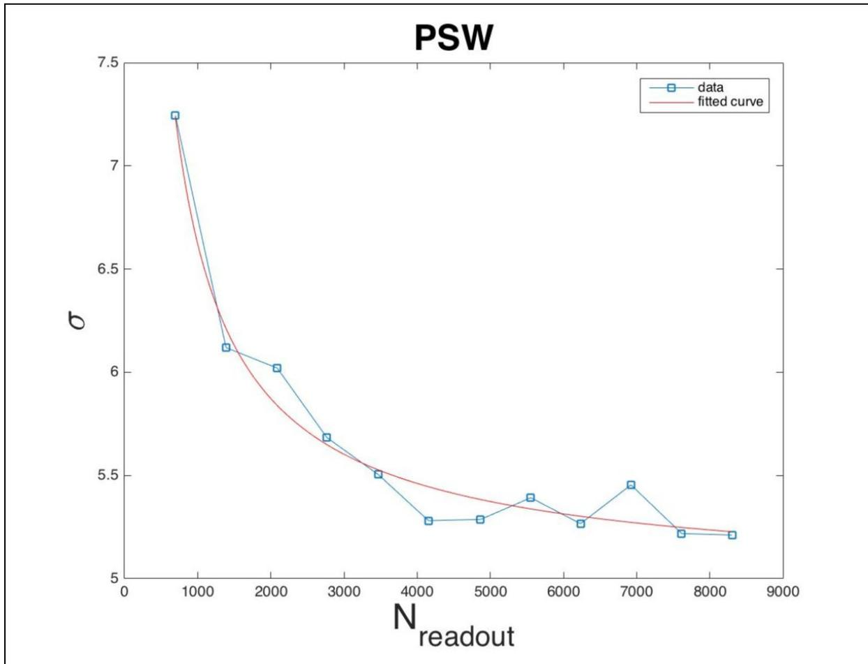
Figure 1.19: The flux uncertainty ( $\sigma$  - standard deviation of the measured flux) values as a function of the average readout number (blue squares). The uncertainty is decreasing according to a power law. The fitted function is shown as a solid red line.
