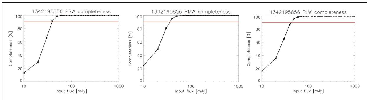
Figure 3.11.: Completeness in the COSMOS field in the PSW, PMW and PLW bands. In all bands the >90% completeness (red solid line) is reached below 50 mJy.
