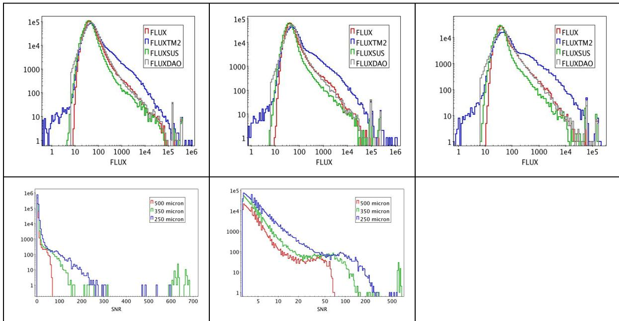
Figure 3.5: Flux distributions for the four different extraction methods. The wavelengths are 250 $\mu$ m, 350 $\mu$ m, and 500 $\mu$ m from left to right. The lower row shows the SNR distributions for all three wavelengths with a linear (left) and a logarithmic (center) x-axis.
