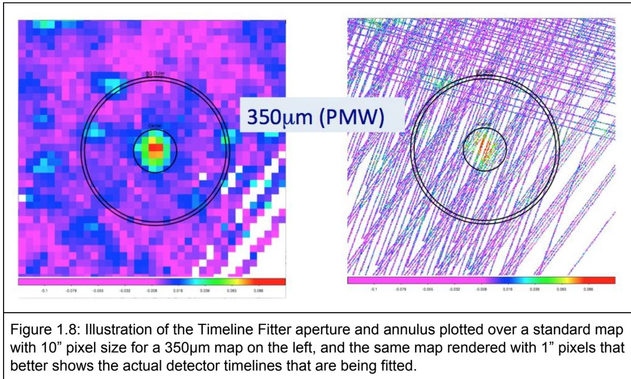
Figure 1.8: Illustration of the Timeline Fitter aperture and annulus plotted over a standard map with 10'' pixel size for a 350µm map on the left, and the same map rendered with 1'' pixels that better shows the actual detector timelines that are being fitted.
