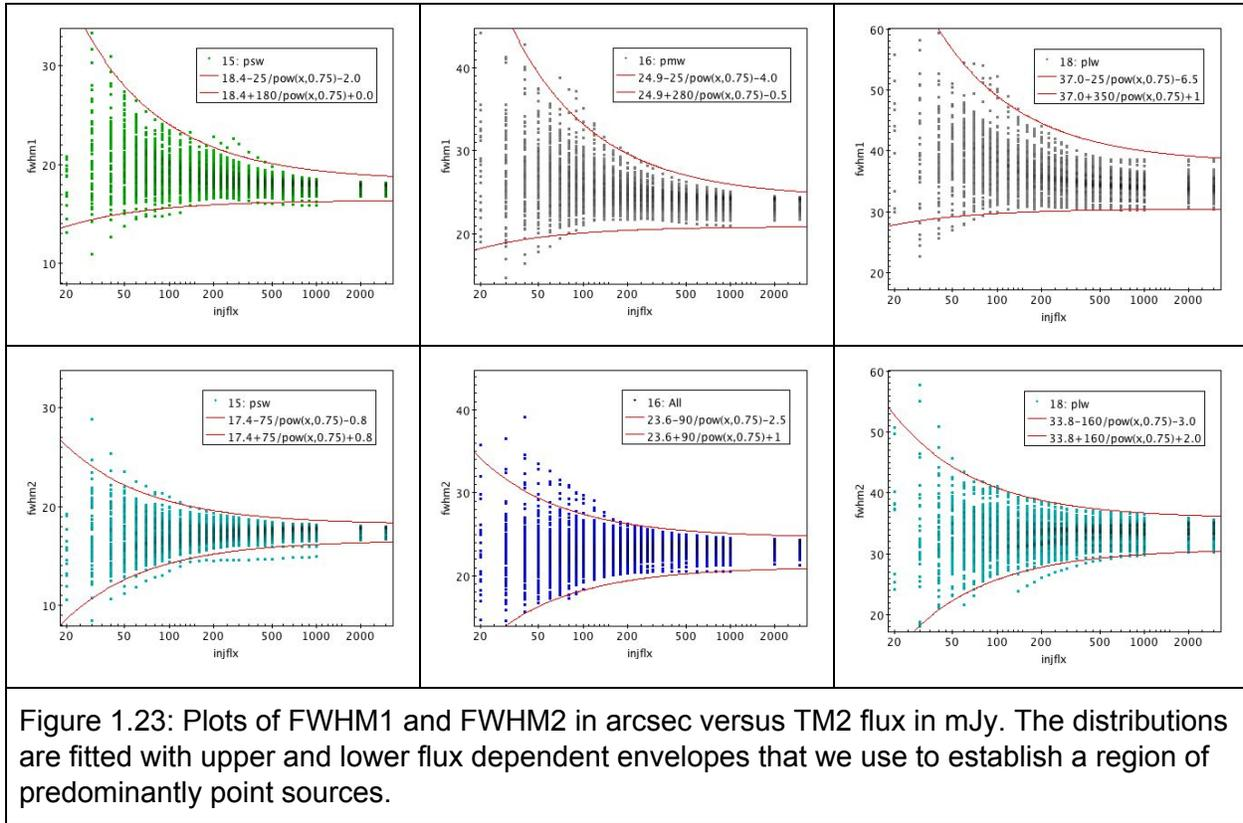
To account for the difference between the injected circular beam profiles and the actual slightly elliptical beam profiles, we corrected the respective functions by adding or subtracting the differences. The actual values for the major and minor axes of the beam profiles are given in Table 1.5 as  $\delta_{0maj}$  and  $\delta_{0min}$ . We then set a point source flag for the major and minor FWHM,  $\delta_{maj}$  and  $\delta_{min}$ , of a given object if the following conditions are satisfied:
