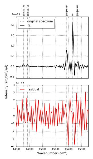
Figure 6. Example of a fit realized wit ORCS (Martin et al. 2015) on a spectrum of a bright region of an HII region in the red SN3 filter. The model used is the convolution of a Gaussian emission line and a sinc ILS (Martin et al. 2016). A modeling error is clearly visible near the right lobe of the emission lines.
