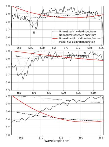
Figure 9. Normalized SITELLE's flux calibration functions. The observed spectrum of the standard star and the standard spectrum are shown. The model calibration function based on our knowledge of the different transmission functions considered in equation 24 is also shown. This model is not used for the calibration.
