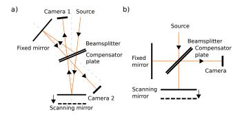
**Figure 1.** a) Sketch of SITELLE's interferometer. b) Sketch of a classical Michelson interferometer.
