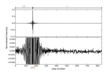
Figure 2. Example of a typical continuum source interferogram obtained with SITELLE. It has been recorded near the center of M31 in the SN3 filter (courtesy of Anne-Laure Melchior). The top panel shows the full interferogram and the bottom panel shows a zoomed version. The ZPD (step 168, indicated with an orange tick) is positioned at the highest measured intensity of the interferogram. The maximum OPD attained on the left side is  $L_1$  and L on the right side (see equations 8 and 9.
