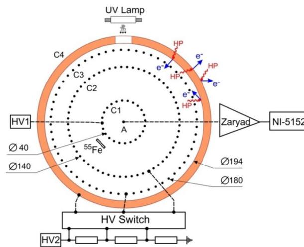
Figure.1. A simplified scheme of a multicathode counter.
