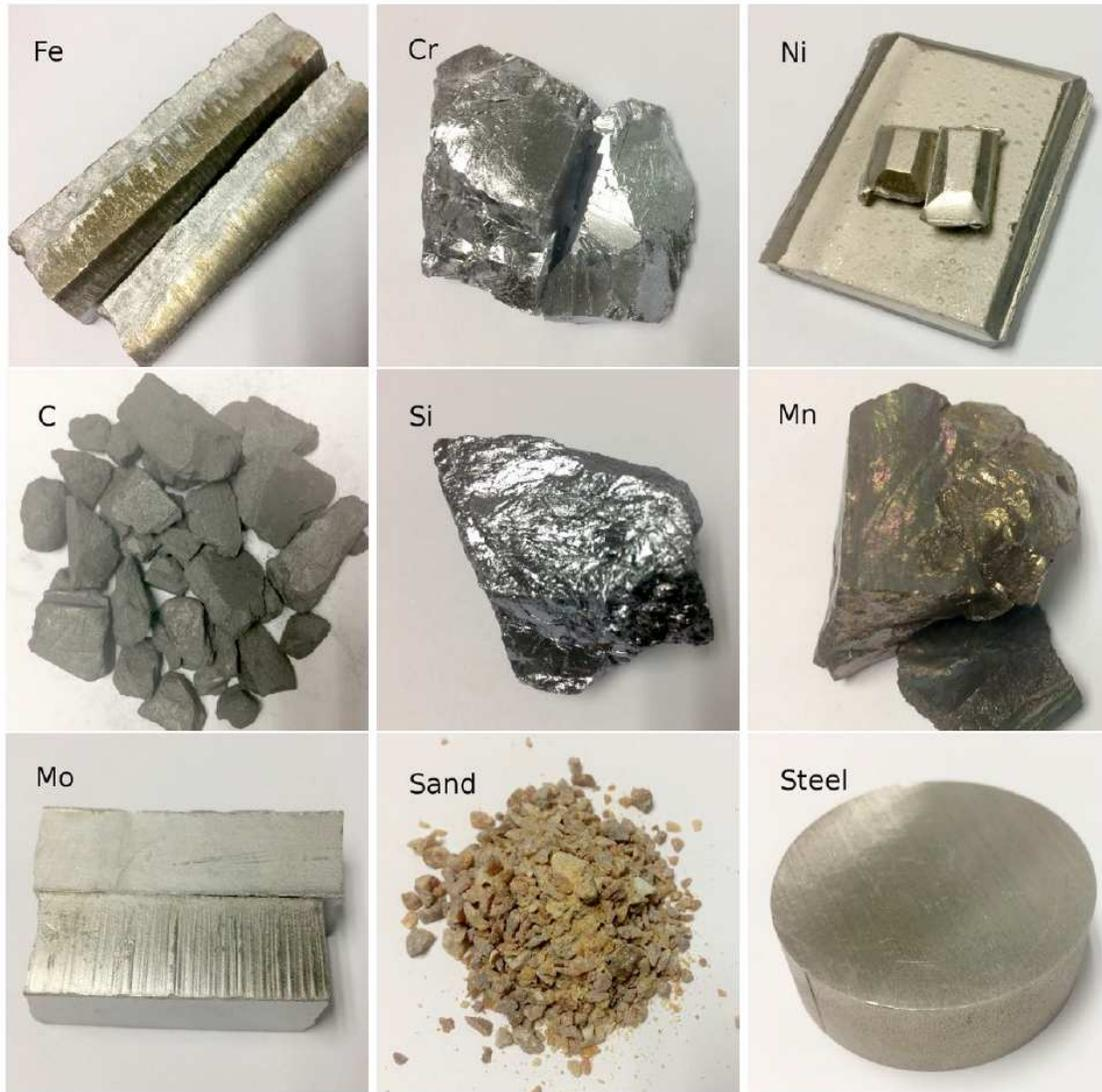
FIG. 1: Raw materials, MgO sand and a SST sample.
