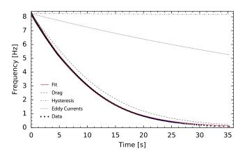
FIG. 8. Spin-down test from 8.5 Hz to 0.2 Hz. Equation 10), which takes into account the three loss mechanisms discussed in Section III D, was fit to the data. The red line is the best-fit model. The gray dashed, dash-dot, and dotted lines represent the three terms of model plotted individually using the best-fit parameters.
