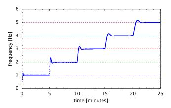
FIG. 6. Rotation frequency as a function of time. The target rotation frequency was changed every 5 minutes. The horizontal dashed lines indicated the target rotation frequencies. After settling, the feedback system successfully maintained the desired rotation frequency. Though the plot shows data for rotation frequencies up to 5 Hz, we tested rotation frequencies up to approximately 10 Hz.
