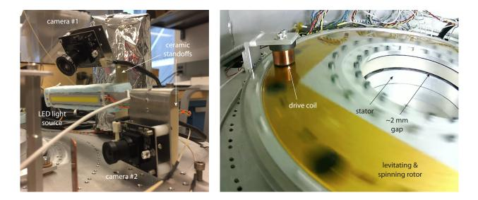
FIG. 5. Left: A photograph of the two cameras that are mounted inside the cryostat. These cameras allowed visual monitoring during 50 K operation. Right: One frame from a movie that was recorded using camera #1. The rotor is levitating and rotating.
