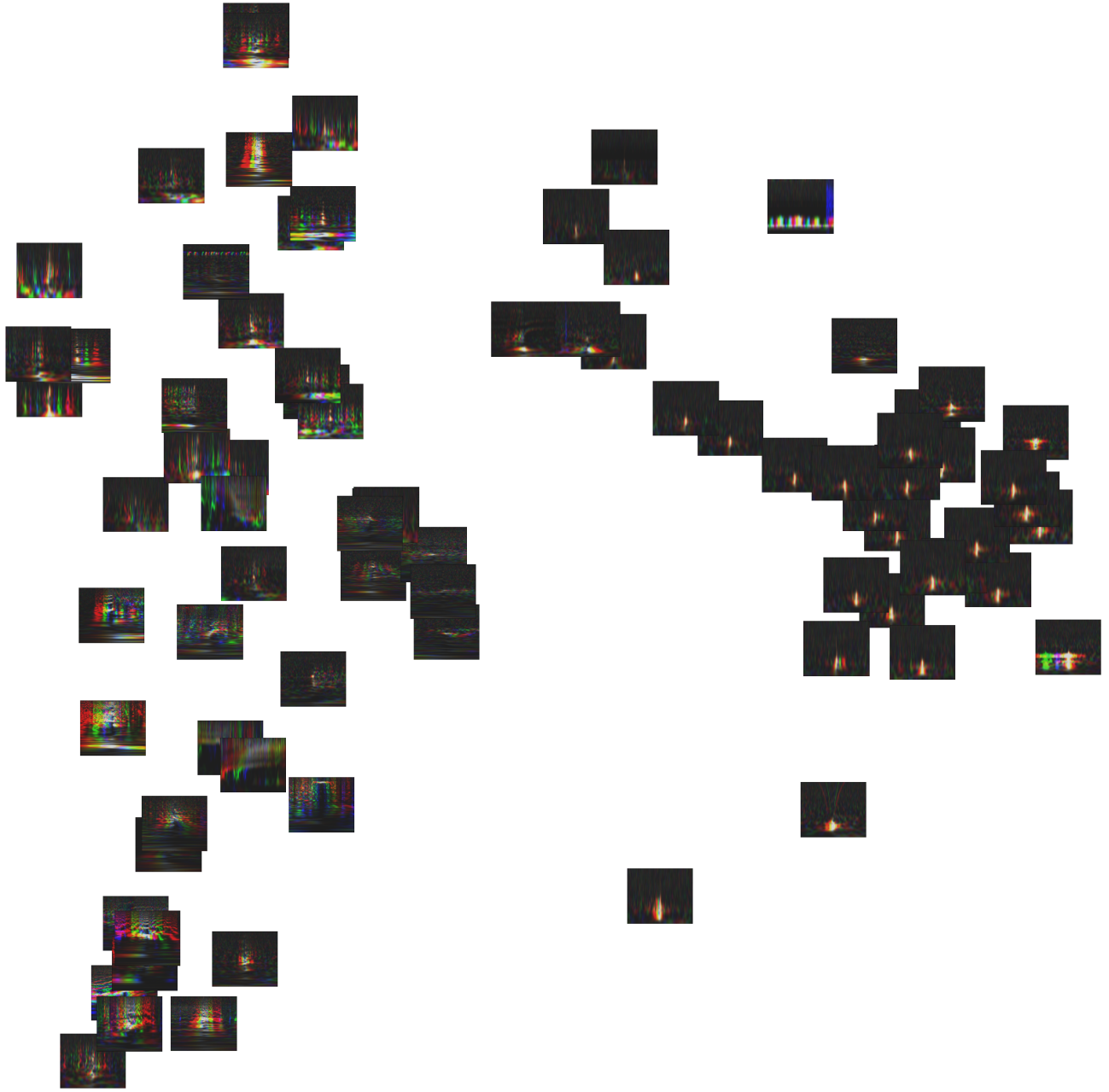
Figure C3: Unsupervised clustering of glitches belonging to none of the known classes. Note that glitches having similar morphology are located near each other. Our trained CNNs were used as feature extractors to map the images to a 1008-dimensional vector-space, which in turn was mapped to the 2-D space shown above using the t-SNE dimension reduction method. This feature-extractor can be used to group new classes of glitches by morphology and find the time of their occurrence in the future.
