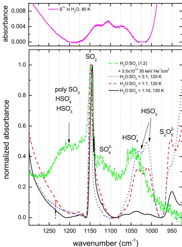
**Fig. 2.** Comparison of the results obtained by three different kinds of ice processing: thermal processing of different H<sub>2</sub>O:SO<sub>2</sub> mixtures, ion bombardment (30 keV He<sup>+</sup>) of the same mixed species, and implantation of S<sup>7+</sup> ions in water ice.
