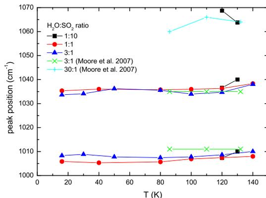
**Fig. 3.** Peak positions of bisulfite ions (HSO<sub>3</sub><sup>-</sup>) in different H<sub>2</sub>O:SO<sub>2</sub> ice mixtures during thermal processing.
