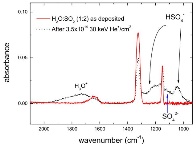
**Fig. 1.** Infrared transmittance spectra of H<sub>2</sub>O:SO<sub>2</sub>=1:2 ice mixture as deposited at T= 16 K and after 30 keV He<sup>+</sup> ion irradiation (the given fluence corresponds to a deposited dose of 12.3 eV/16 u). We note that the broad band around 1200 cm<sup>-1</sup> is due to more than one species, including SO<sub>3</sub> sulfur polymers (see Table 2).
