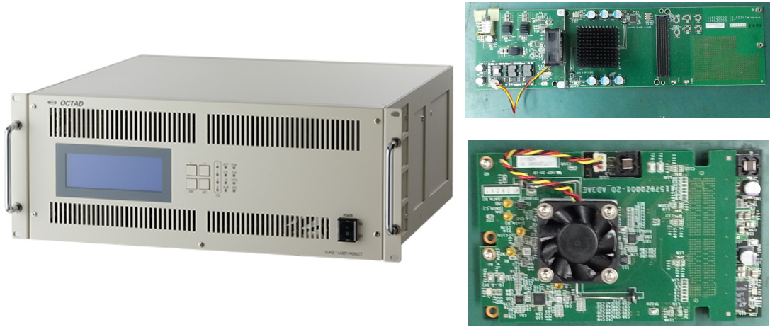
Figure 1. Photographs of the OCTAD-S. (Left) Overview of the instrument. (Upper right) DSP module and (lower right) ADC module.
