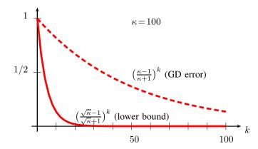
**Fig. 4.** Upper bound (28) on convergence rate of GD and lower bound (30) on convergence rate for any FOM minimizing functions  $f(\cdot) \in S_n^{L,U}$  with condition number  $\kappa = U/L = 100$ .
