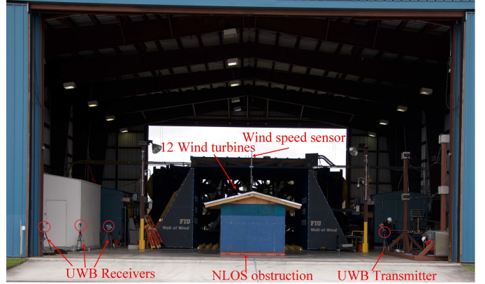
Fig. 1. UWB channel measurement setup at Florida International University, Wall of Wind facility, Miami, FL.
