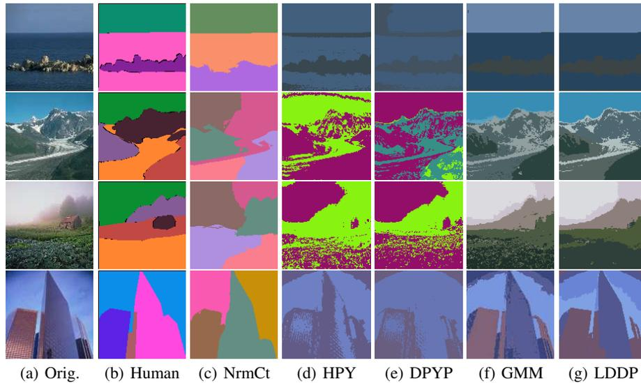
**Fig. 4.** Example segmentations when ground truth is known. The number of clusters is set to ground truth for all experiments to facilitate a head-to-head comparison of the modeling structure. LDDP performs better than other Bayesian methods and comparable to normalized cuts. We see the improvement of LDDP over GMM as a result of the added Gaussian processes.
