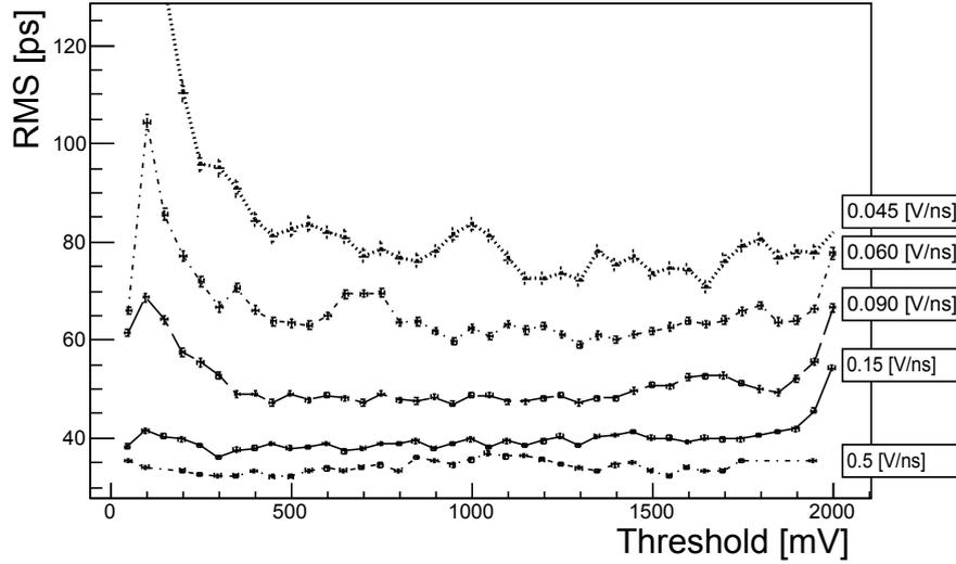
**Figure 5.** The average precision of the time difference measurement as a function of a threshold level and slew rate.
