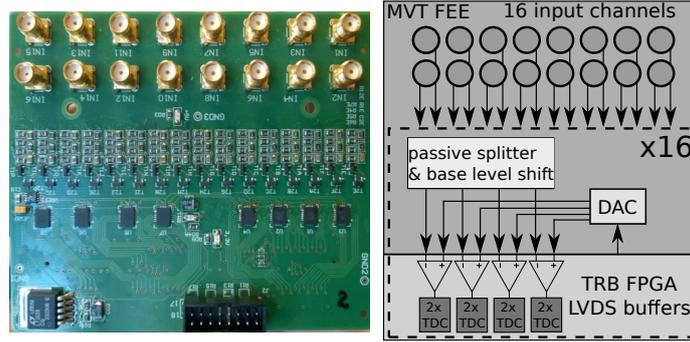
**Figure 2.** Picture of the MVT mezzanine card (left) and block diagram which represents its functionality (right). The MVT board has 16 channels where analogue signals are split into four with passive splitters and together with threshold voltage signals generated by DAC are passed to the FPGA LVDS buffers.
