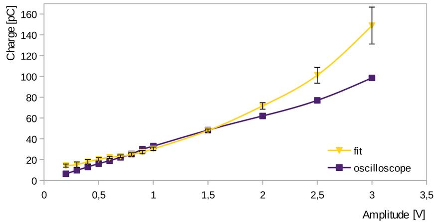
**Figure 4.** The charge of the signal as a function of the amplitude. Triangles denote the charge (before splitting) reconstructed using the method described in the text, and squares indicate the charge measured using the Serial Data Analyzer (Lecroy SDA6000A).
