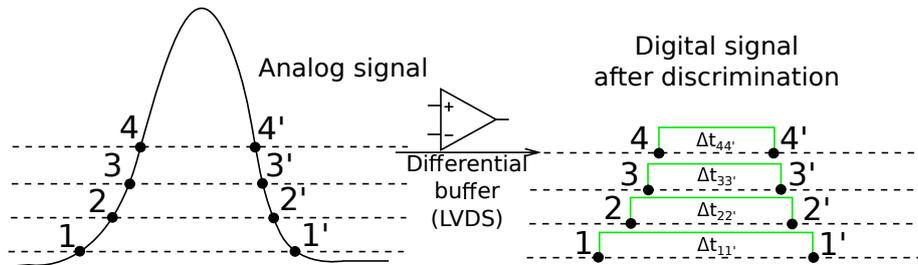
**Figure 3.** The method of signal sampling described in this article. Sampling on different voltage levels allows to determine more precisely the start time of the signal and its charge. It may be done by fitting a curve which describes the shape of the signal using either the method of library of synchronised model signals [9] or by more advanced methods as e.g. the signal shape reconstruction by means of the compressive sensing theory [10, 11].
