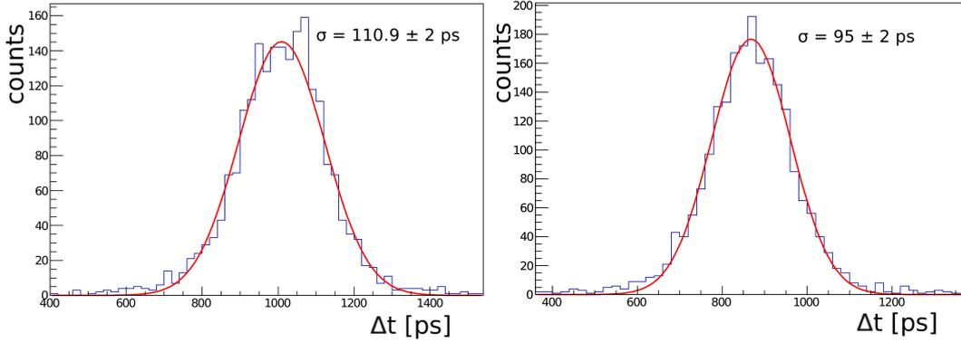
**Figure 8.** Distribution of the difference between times recorded at the lowest threshold for the rising edge of signals from the left and right photomultipliers. Before (left) and after (right) time walk correction.
