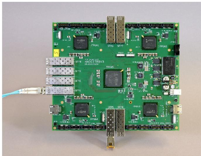
**Figure 1.** The TDC Readout Board (TRB) consists of the control FPGA placed in the centre and other four FPGA's providing 196 TDC channels. On the edges of the board high data rate connectors are located to directly measure signals or to attach mezzanine cards.
