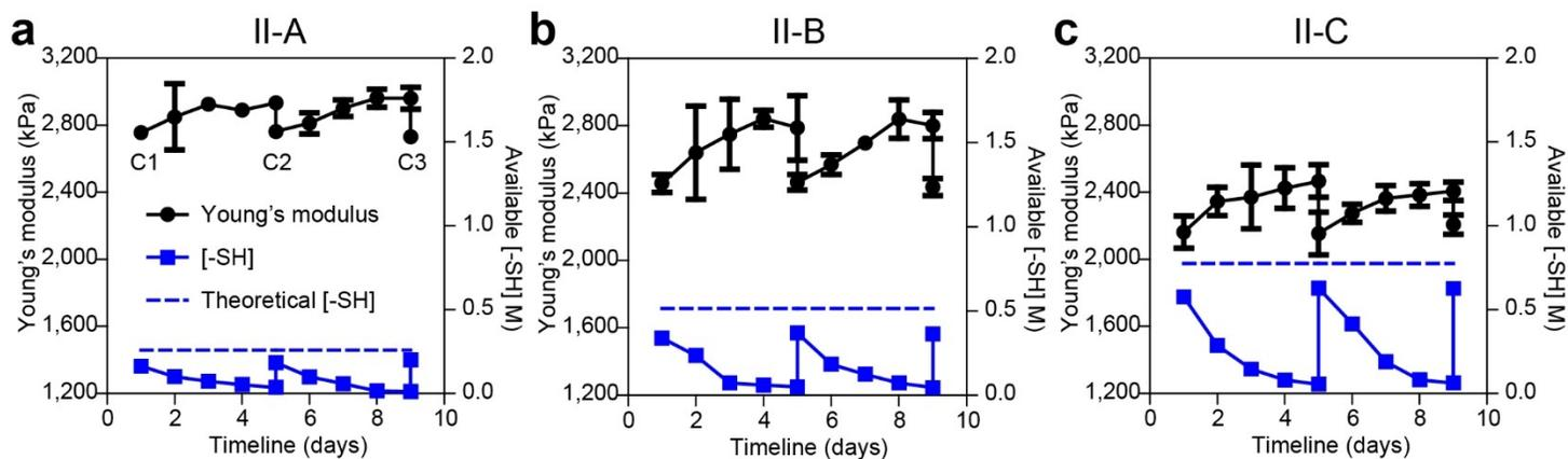
**Figure 3 | Reversibility of latent thiol crosslinking.** a-c, Recovery of thiols (blue) and Young's modulus (black) over three oxidation-reduction exchange reactions from Set II with different gel compositions. Cycles 1, 2, and 3 started on Days 1, 5, and 9, respectively. a, II-A (low [-SH]). b, II-B (intermediate [-SH]). c, II-C (high [-SH]).
