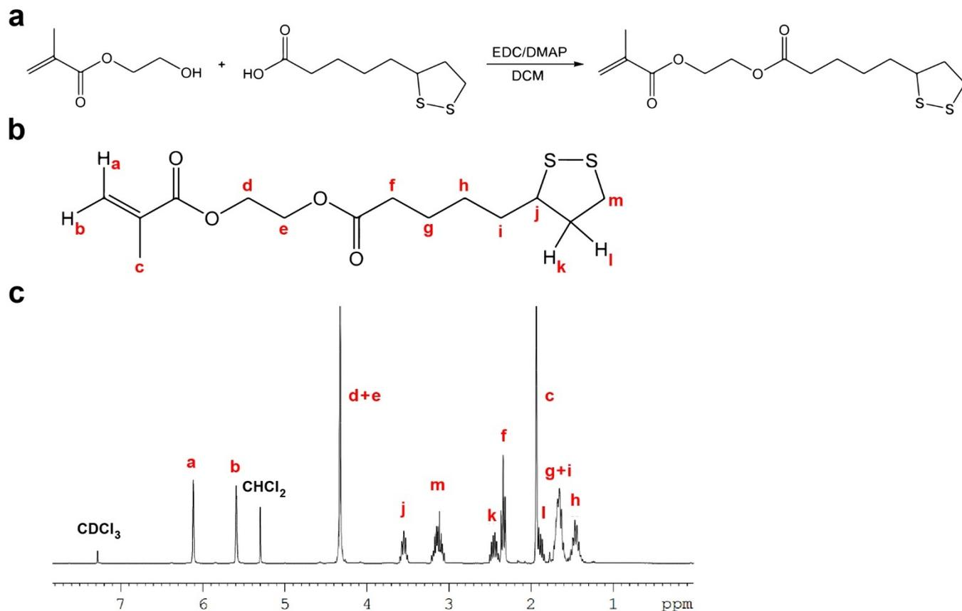
**Supplementary Figure 1 | Synthesis of HEMA-LA.** a, Homopolymerization of HEMA-LA by RAFT reaction between HEMA and LA using EDC as coupling agent and DMAP as catalyst in DCM. b, Chemical structure of HEMA-LA. c,  $^1\text{H}$  NMR spectrum of HEMA-LA.
