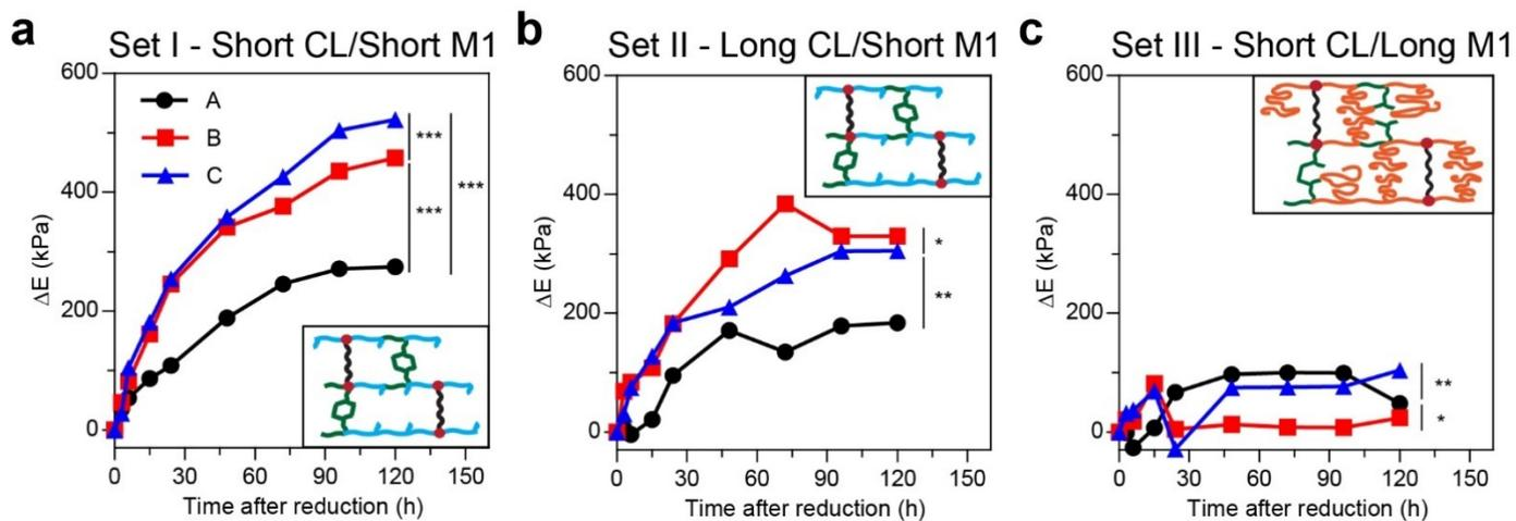
**Figure 4 | Shielding effect on gel stiffening via long dangling monomers. a-c,** Change in Young's modulus  $\Delta E$  over time post-reduction of different gel structures. **a,** Set I (short CL/short M1). **b,** Set II (long CL/short M1). **c,** Set III (short CL/long M1). Insets: schematics of disulfide formation in gel network during oxidation.
