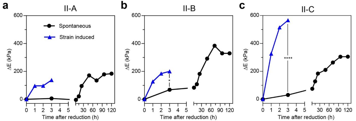
**Figure 5 | Strain-induced latency of intermolecular disulfide crosslinks. a-c,** Change in Young's modulus post-reduction under strain (blue) for 3 hours compared to spontaneous state (black) using Set II. **a,** II-A (low [-SH]). **b,** II-B (intermediate [-SH]). **c,** II-C (high [-SH]).
