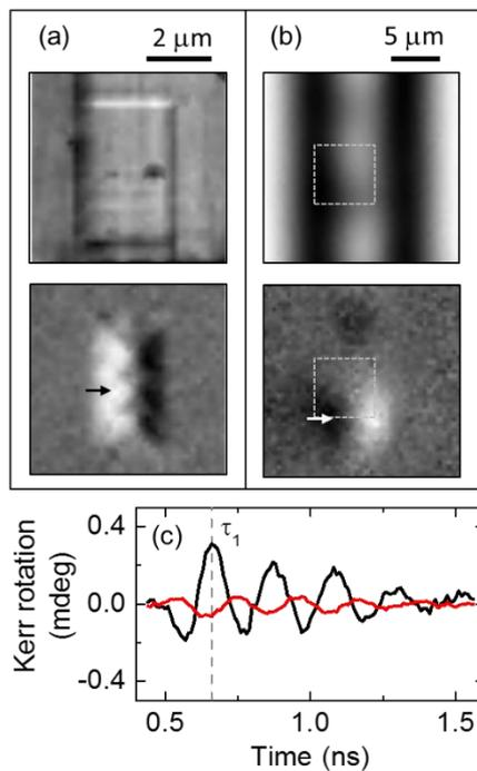
Figure 6. Images of reflectivity (top) and polar Kerr rotation (bottom) are shown for near-field TRSKM in (a) and TRSKM using the  $\times 8$  microscope objective of the LensAFM in (b). The near-field image range is indicated by the grey dashed square in (b), while the arrows in the polar Kerr images indicated the location at which the time-resolved traces in (c) were acquired.
