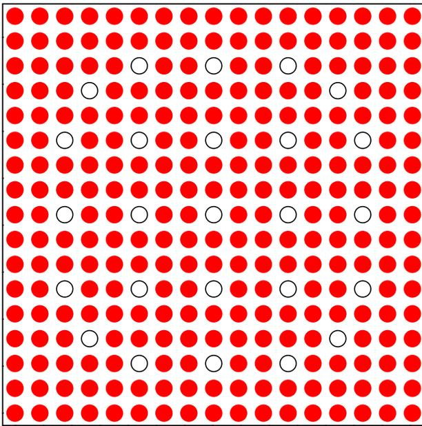
**FIGURE 1.** 17x17 PWR lattice configuration
