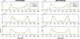
Fig. 1. Scatter profiles from the CNN and from MC (as ground truth) at the center slice for three different views (from top to bottom). X axis is downsampled detector line; y axis is normalized scatter intensity.
