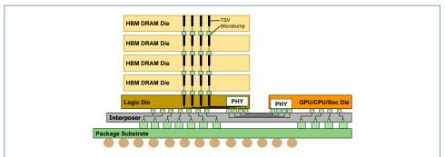
Figure 5: 3D-Stacked DRAM example: High Bandwidth Memory consists of stacked memory layers and a logic layer connected by high bandwidth TSVs and microbumps [7]. The 3D-stacked memory is then connected to an SOC with an interposer layer that provides high bandwidth between the logic layer and the processing units on the package substrate.
