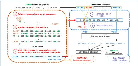
Figure 3: Flow diagram for our algorithm. GRIM-Filter takes in read sequences and generates filter masks on the 3D-stacked logic die using precomputed bit vectors, while the CPU filters locations, queried from the hash table, using the resulting filter mask. The locations of correct mappings and their edit distances are then returned to the user.
