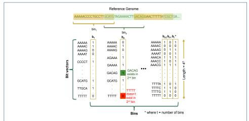
Figure 2: Data structure layout of bit vectors. Columns are indexed by bin-number-converted locations. Rows are indexed by the token hash value. In this figure, token size=5.
