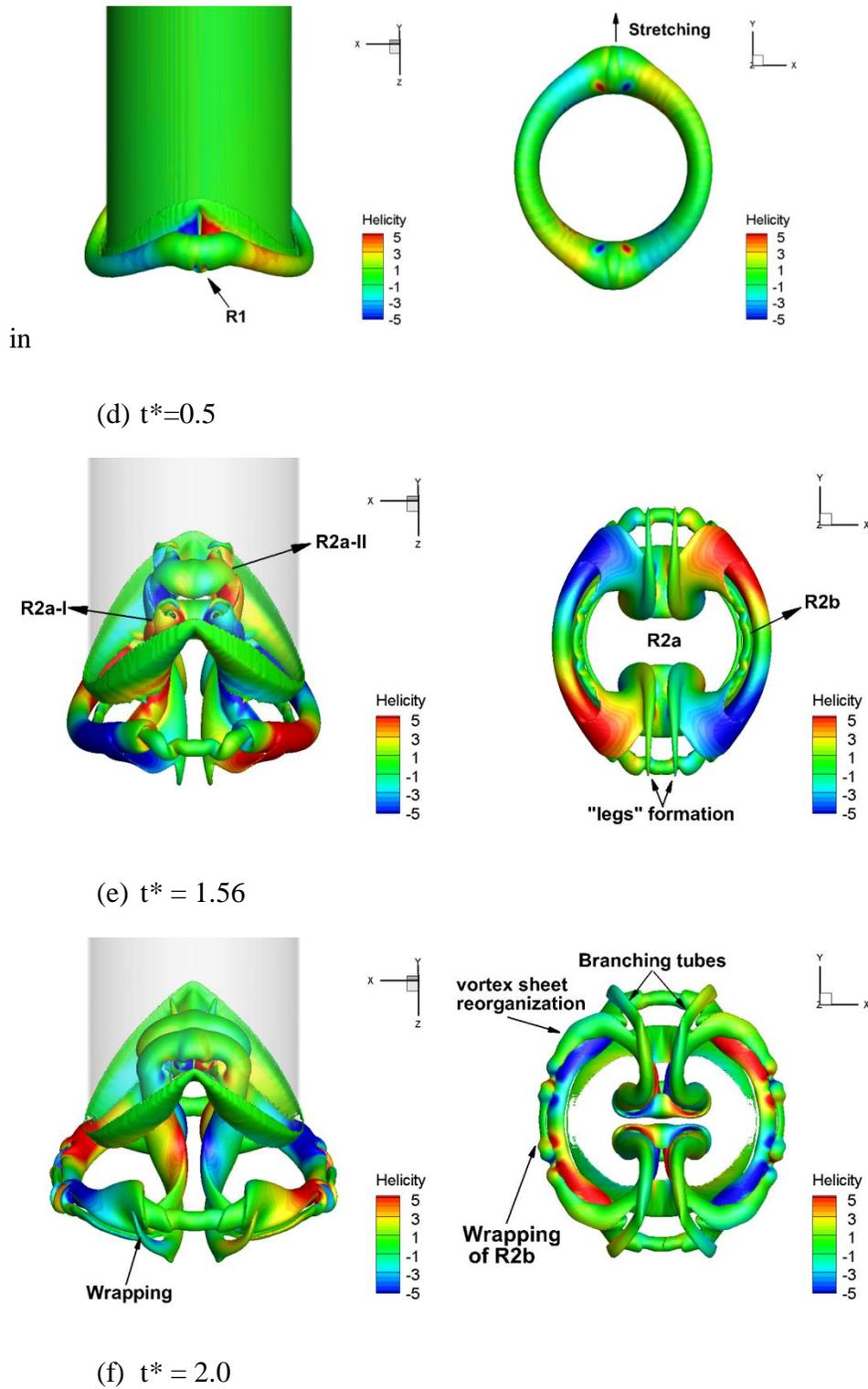
Figure 10a. There exists a primary vortex core ( $R1$ ) following the shape of V-shape exit closely. Similar to A-notched nozzle, the core's size in this case also continuously varies along the
