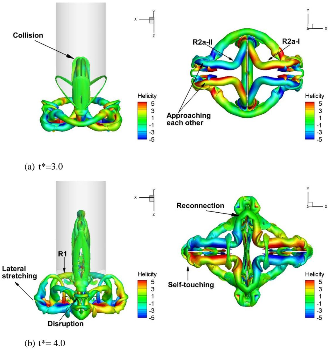
Figure 9: The collision of two secondary rings in A-notched nozzle are visualized by iso-surface of vorticity magnitude colored by helicity density. The spanwise vortices are formed at peaks while streamwise vortices at troughs are remaining parts of secondary rings
