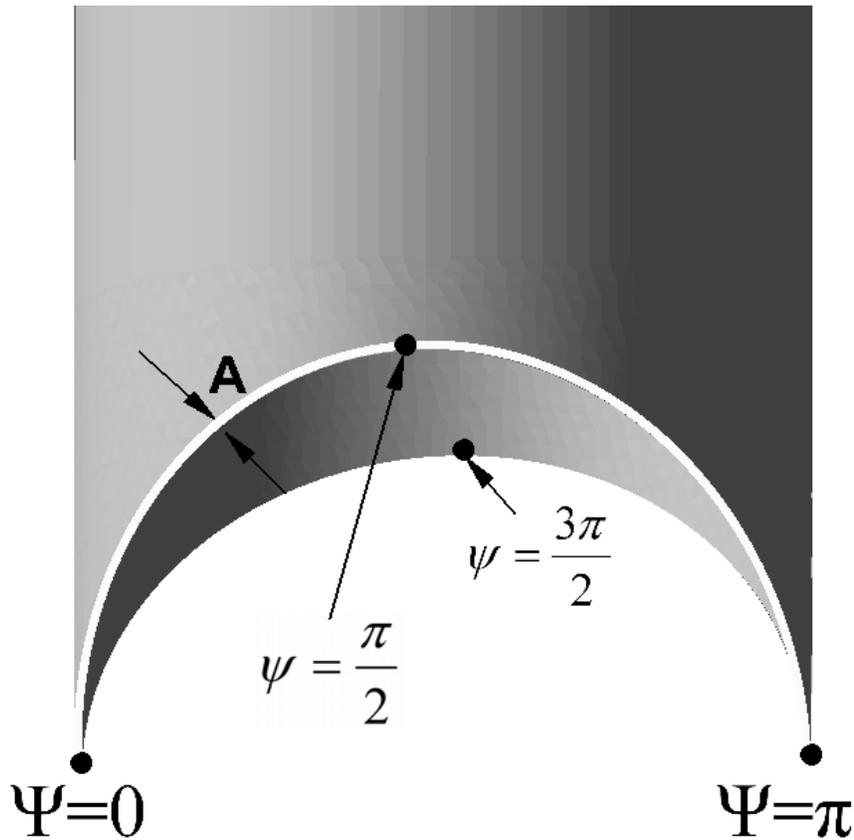
Figure 2 The close-up view for the exit of A-notched nozzle. The longest lip of nozzle is marked with  $\psi=0$ . The plane *peak-to-peak* is defined as the plane cut through locations of  $\psi=0$  and  $\psi=\pi$ . The *trough-to-trough* plane is the plane of  $\psi= \pi/2$  and  $\psi=3\pi/2$ . The thickness of the nozzle is denoted as  $A=1.78$  mm.
