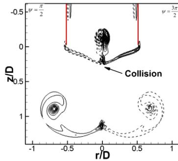
Figure 7: The vorticity fields at the exit of V-notched nozzle at different instances depict the formation of the primary ring as well as the collision of trailing rings. Left column is displayed in *peak-to-peak* plane which is orthogonal to the *trough-to-trough* plane (right column). The first contour level is  $2.5$  with the increment is  $2.5DU_0$ . The dash lines indicate negative values.
