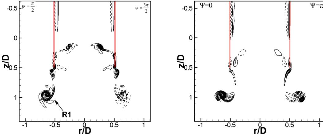
Figure 13 The vorticity fields at the exit of W-notched nozzle at  $t^* = 2.62$  depicting the formation of the primary ring. Left column is displayed in *sharp peak-to-sharp peak* plane which is orthogonal to the *round peak-to-round peak* plane (right column). The first contour level is 2.5 with the increment is  $2.5DU_0$ . The dash lines indicate negative values.
