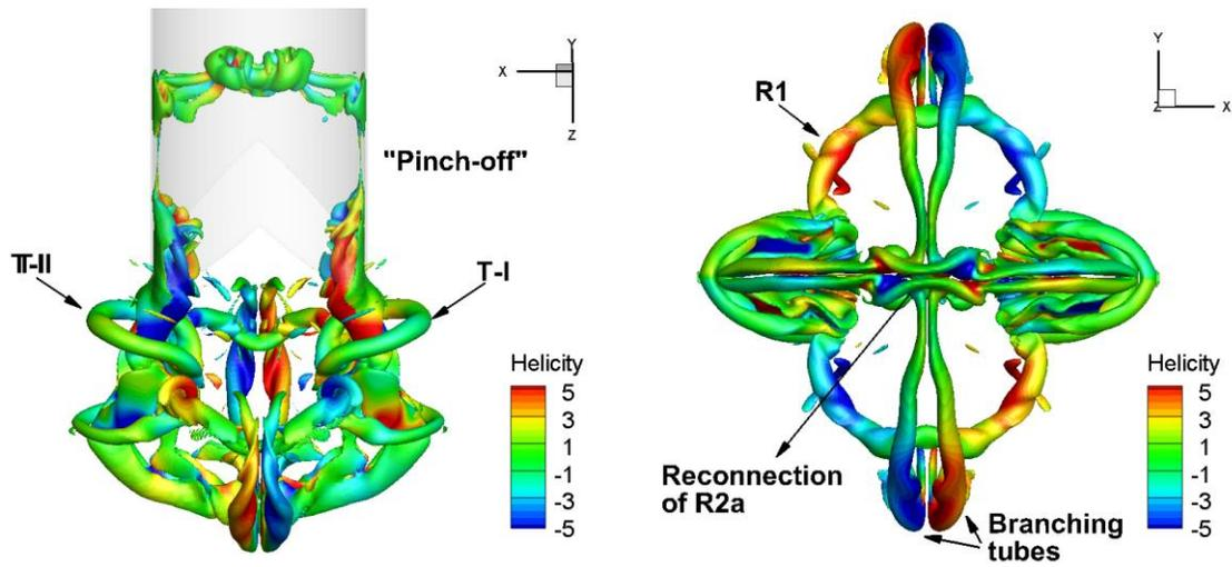
Figure 12: The collision of two secondary rings in V-notched nozzle are visualized by iso-surface of vorticity magnitude colored by helicity density. The spanwise vortices are formed at peaks while streamwise vortices at troughs are remaining parts of secondary rings at  $t^*=4.0$
