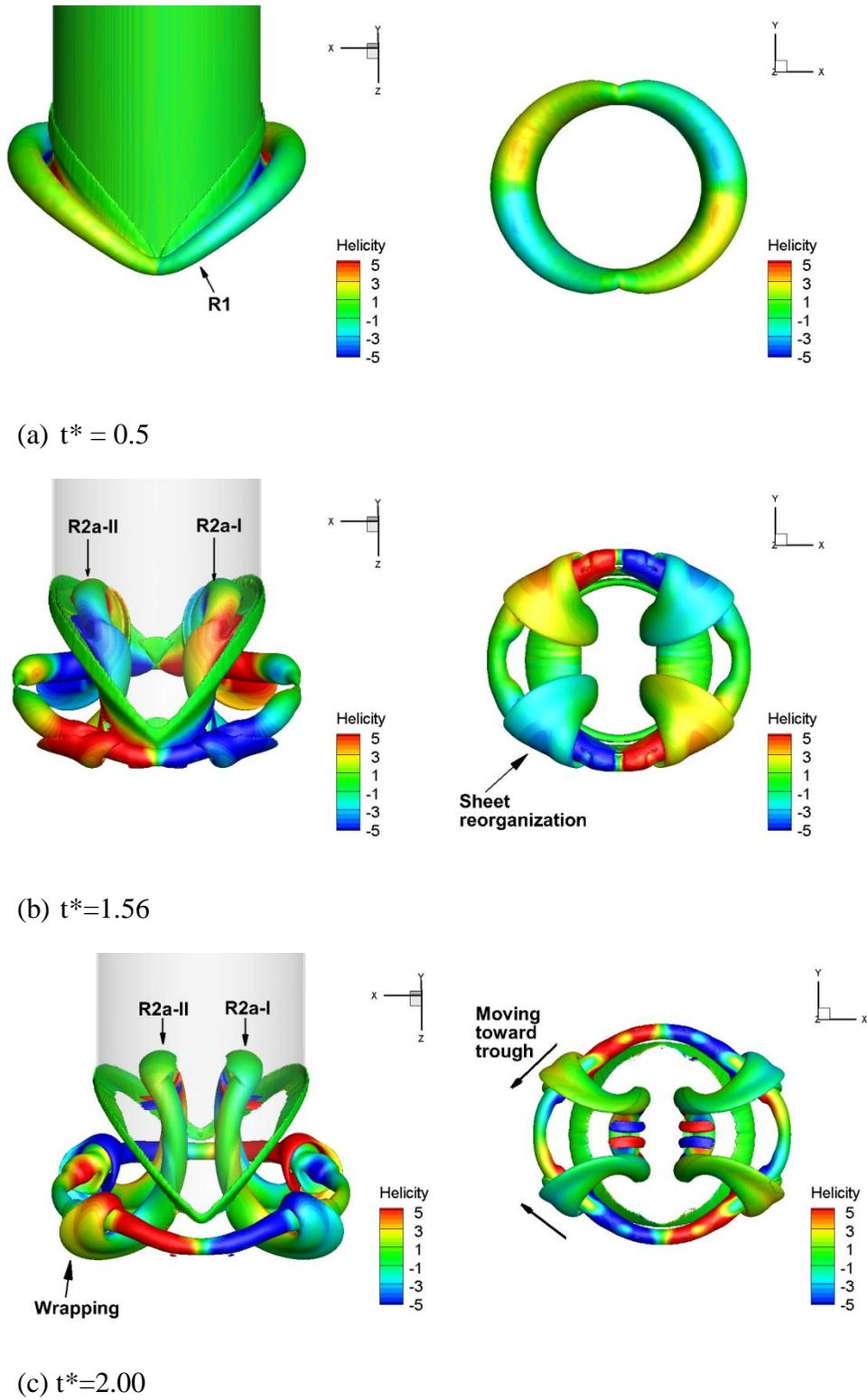
Figure 8: The evolution of vortex ring interaction is visualized by vorticity magnitude colored by helicity density for A-notched nozzle. Each column displays the side view and bottom view at the same time instance. From left to right, the column display the time:  $t^*=0.5$ ,  $t^*=1.56$  and  $t^*=2.00$ . The primary ring (R1) is formed following the A-shape of the exit. Two distinct trailing rings (R2a-I and R2a-II) are created at trough locations after the piston stops.
