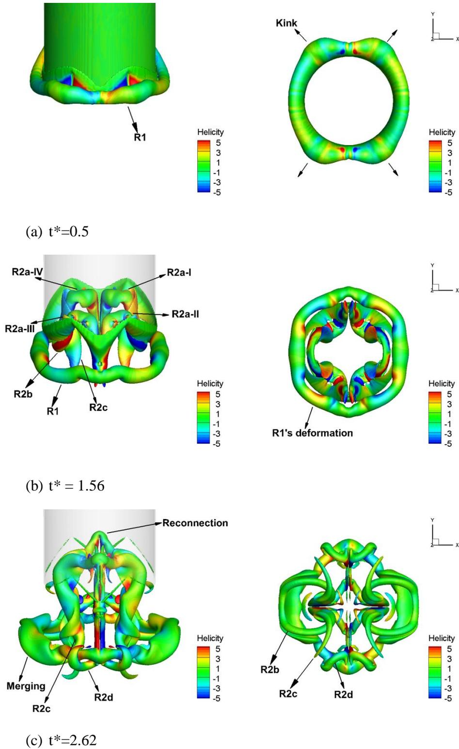
Figure 14: The evolution of vortex ring interaction is visualized by vorticity magnitude colored by helicity density for W-notched nozzle. Each column displays the side view and bottom view at the same time instance. From left to right, the column display the time:  $t^* = 0.5$ ,  $t^* = 1.56$  and  $t^* = 2.62$ .
