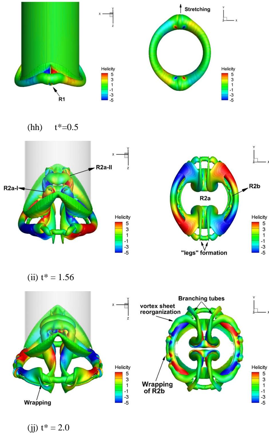
Figure 10 from a-c shows that the discontinuity (sharpness) of the exit at peaks in A-notched nozzles regulates the interruption of the vortex sheet's rolling-up at peaks. The vortex sheet is
