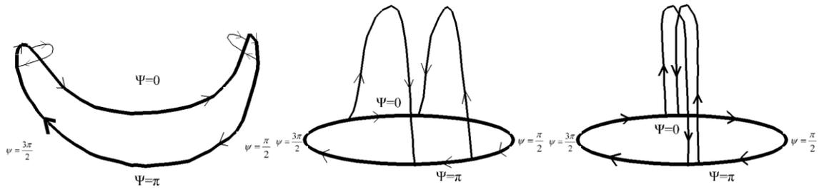
**Figure 15: The vortex structure of the asymmetrical ring from notched nozzle. The lines indicate the vortex line and the arrow indicates the vorticity vector direction.**
