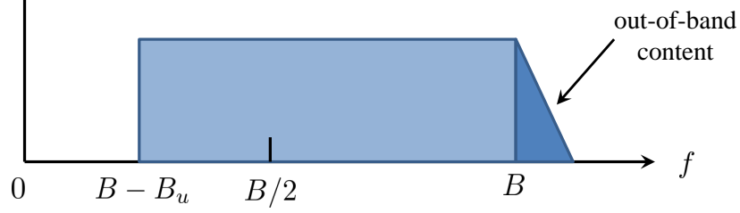
Fig. 3: A non-ideal relay filter results in some residual out-of-band content.
