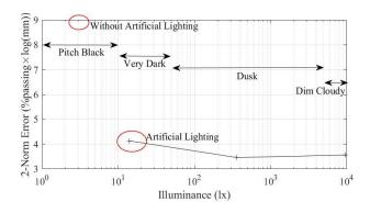
Figure 6: 2-norm error between the estimated rock size distributions and the sieve analysis reference curve plotted against illuminance measurements for outdoor experiments. Qualitative measures of common lighting conditions are provided as ranges of illuminance measurements.
