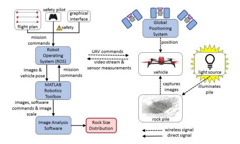
Figure 1: Block diagram of the aerial vehicle system used for aerial fragmentation analysis. Arrows show the typical information flow while conducting a flight plan.
