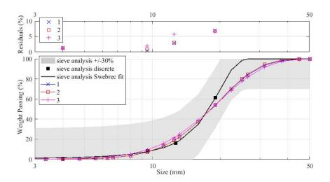
Figure 5: Rock fragmentation analysis results for lab experiments with respect to the sieve analysis reference curve. Discrete points represent the combined results for each set of images collected during each experiment. The gray envelope represents the accepted maximum error envelope of 30% recommended by [4] for industry standard 2D image analysis.
