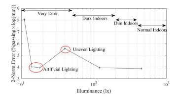
Figure 4: 2-norm error between the estimated rock size distributions and the sieve analysis reference curve plotted against illuminance measurements for indoor experiments. Qualitative measures of common lighting conditions are provided as ranges of illuminance measurements.
