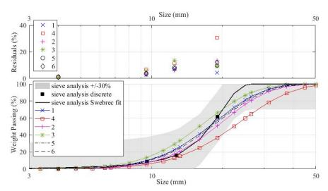
Figure 3: Rock fragmentation analysis results for indoor experiments with respect to the sieve analysis reference curve. Discrete points represent the combined results for each set of images collected during each experiment. The gray envelope represents the accepted maximum error envelope of 30% recommended by [4] for industry standard 2D image analysis.
