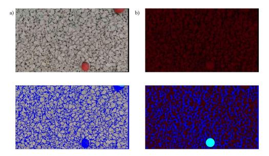
Figure 2: a) Raw and delineated photo captured in ideal lighting (450 lx). b) Raw and delineated photo captured in dark conditions (11 lx).
