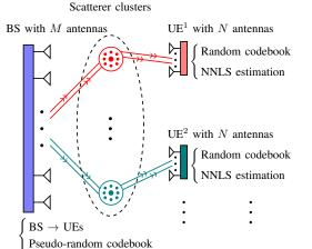
Fig. 1: Illustration of the physical channel model and our proposed Beam Alignment (BA) scheme.
