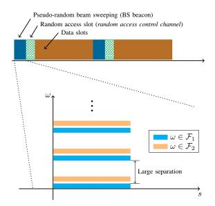
Fig. 3: (Top) Frame structure of the proposed BA scheme. (Bottom) Different beacon signals are orthogonally multiplexed over disjoint sets of subcarriers  $\omega \in \mathcal{F}_i$ ,  $i \in [m]$ . In the figure's example we have two orthogonal beacon signals on the "blue" and on the "orange" combs of subcarriers.
