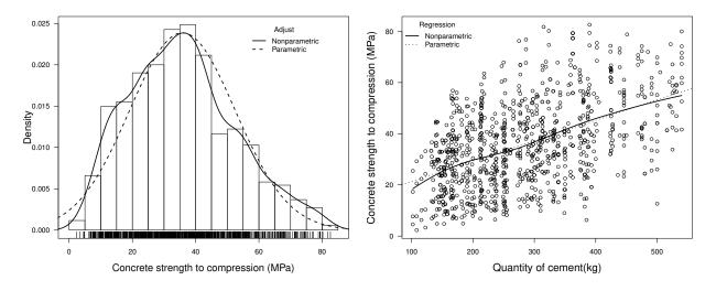
Figure 3: Histogram and scatter plot for concrete strength.
