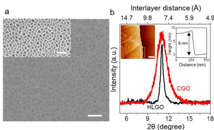
**Figure 1| Ultrathin HLGO membrane.** (a) SEM image of an 8 nm thick HLGO membrane on an Anodisc alumina support. Scale bar, 1  $\mu\text{m}$ . Inset: SEM image of bare alumina support. Scale bar, 500 nm. (b) X-ray diffraction for HLGO and CGO membranes. Inset (left): AFM image of HLGO membrane transferred from an alumina substrate to a silicon wafer. Scale bar, 500 nm. Inset (right): The height profiles along the dotted rectangle.
