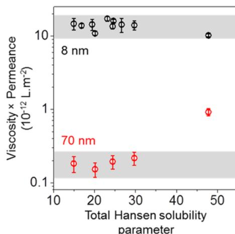
**Supplementary Fig. 10| Probing influence of solubility parameter of solvents on permeation.** Product of permeance and viscosity of solvents as a function of the total Hansen solubility parameter for 8 nm and 70 nm thick HLGO membrane (colour coded). Variations between the points in the grey colour marked region are minor and within the accuracy of measurements. All the error bars are standard deviations using at least three different measurements using different samples.
