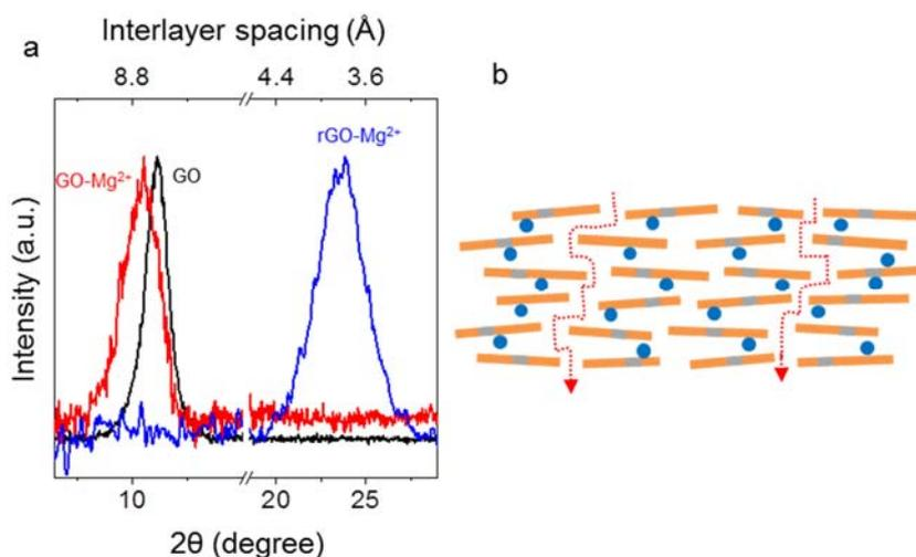
**Supplementary Fig. 11| Mg<sup>2+</sup> crosslinked GO membranes.** (a) X-ray diffraction for pristine GO, Mg<sup>2+</sup> crosslinked GO (GO-Mg<sup>2+</sup>) and partially reduced Mg<sup>2+</sup> crosslinked GO (rGO-Mg<sup>2+</sup>) membranes. The thickness of membranes  $\approx$  200 nm. (b) Schematic showing the structure of the GO-Mg<sup>2+</sup> membrane. The dotted line indicates the permeation pathway and blue circles indicate Mg<sup>2+</sup> ions.
