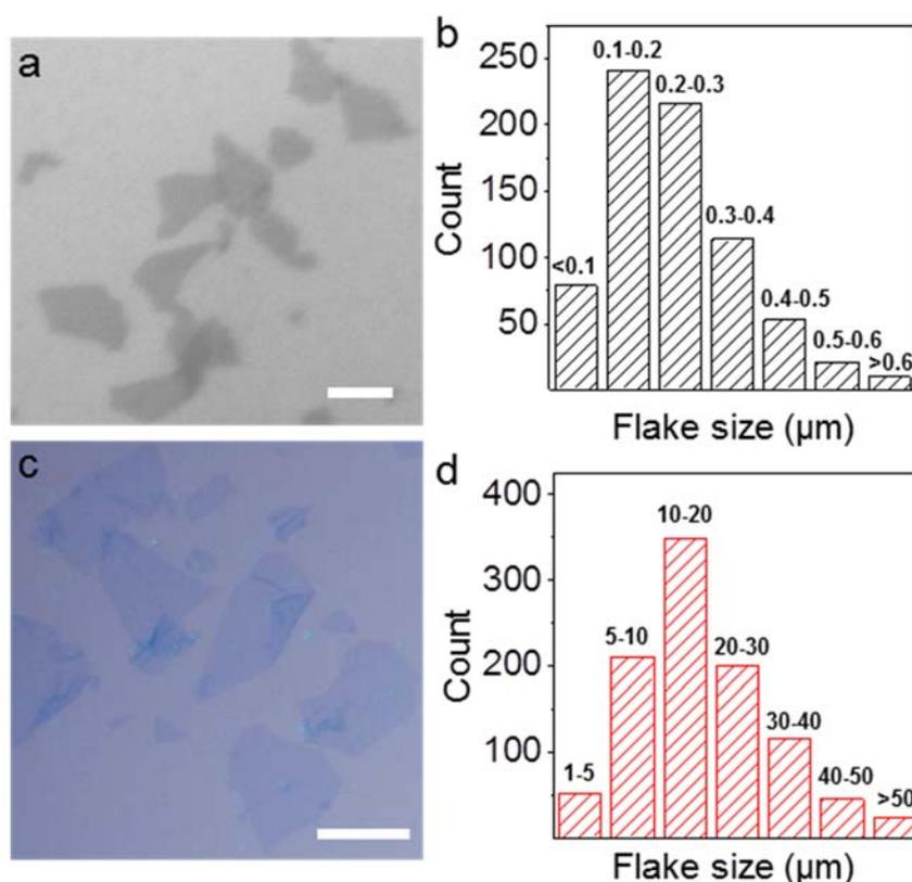
**Supplementary Fig.1| GO flake size distribution.** (a) SEM image of GO flakes used for the preparation of CGO membranes (Scale bar, 200 nm) and (b) its flake size distribution. (c) Optical image of GO flakes used for the preparation of HLGGO membranes (Scale bar, 20 μm) and (d) its flake size distribution. The flake sizes were estimated by taking the square root of the area of each flake measured with the Image J software.
