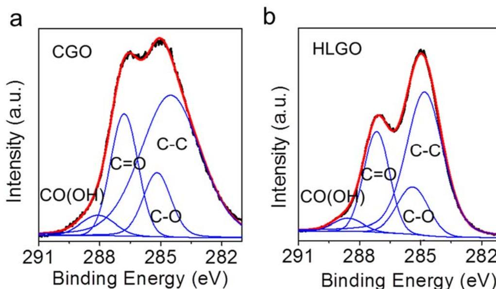
**Supplementary Fig.2| X-ray photoelectron spectroscopy of CGO and HLGO membrane.**
