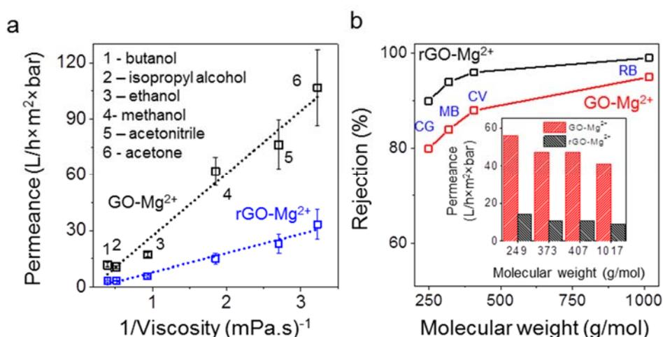
**Supplementary Fig. 12| Permeation through 200 nm thick Mg<sup>2+</sup>-crosslinked GO membranes.** (a) Permeance of various organic solvents through GO-Mg<sup>2+</sup> and rGO-Mg<sup>2+</sup> membrane as a function of their inverse viscosity. The used solvents are numbered and named on the top left. Dotted lines are the best linear fit. (b) Rejection of several dyes in methanol versus their molecular weight. The dyes used: CG, MB, CV, and RB. Inset: The corresponding permeance of methanol.
