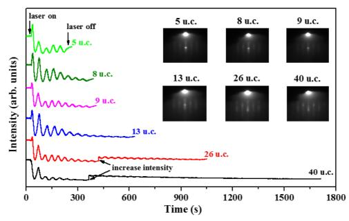
Figure 1. RHEED oscillations recorded during the growth of  $La_{0.9}Ba_{0.1}MnO_3$  films with a thickness from 5 to 40 unit cells. The insets display the RHEED diffraction patterns after the growth.
