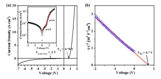
Figure 3. (a) Rectifying current density-voltage (The inset shows the corresponding current density-voltage in semi-logarithmic scale.) and (b) capacitance-voltage characteristics of  $La_{0.9}Ba_{0.1}MnO_3/Nb$ : SrTiO<sub>3</sub> heterojunctions at room temperature for the thickness of 40 unit cells.
