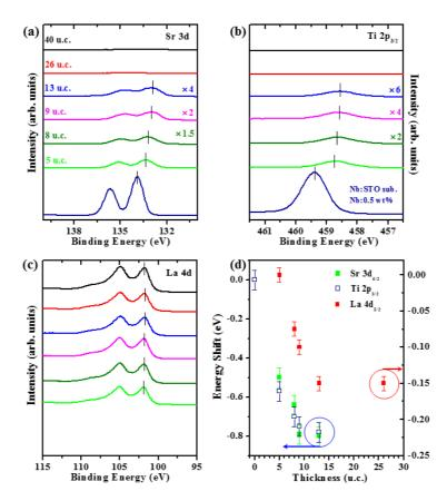
Figure 4. La<sub>0.9</sub>Ba<sub>0.1</sub>MnO<sub>3</sub>-overlayer-thickness dependence of Sr 3d (a) and Ti  $2p_{3/2}$  (b) core-level spectra of buried TiO<sub>2</sub>-terminated Nb-doped SrTiO<sub>3</sub>, (c) La 4d core-level spectrum. (d) Plot of the binding energy shift of the Sr  $3d_{5/2}$ , Ti  $2p_{3/2}$ , and La  $4d_{5/2}$  core-level peaks as a function of the La<sub>0.9</sub>Ba<sub>0.1</sub>MnO<sub>3</sub> overlayer thickness.
