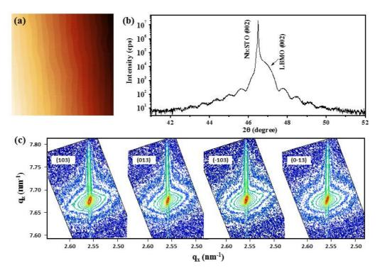
Figure 2. Structural characterization of  $La_{0.9}Ba_{0.1}MnO_3$  film grown on TiO<sub>2</sub>-terminated Nb: SrTiO<sub>3</sub> (001) with a thickness of 40 unit cells: (a) A typical 5 × 5  $\mu$ m AFM height image. (b) XRD  $\theta$ -2 $\theta$  detailed scan around (002) reflection. (c) Reciprocal space maps of (103), (013), (10-3), and (0-13) Bragg reflections of Nb: SrTiO<sub>3</sub> and La<sub>0.9</sub>Ba<sub>0.1</sub>MnO<sub>3</sub>.
