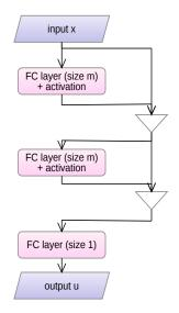
Figure 6: Network structure used for the eigenvalue problem. There are skip connections between every pairwise layers. The triangles denote concatenation operations.
