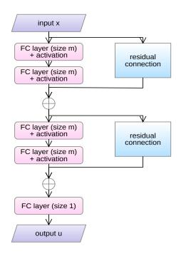
Figure 1: The figure shows a network with two blocks and an output linear layer. Each block consists of two fully-connected layers and a skip connection.
