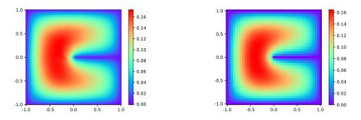
(a) Solution of Deep Ritz method, 811 parameters (b) Solution of finite difference method, 1,681 parameters
