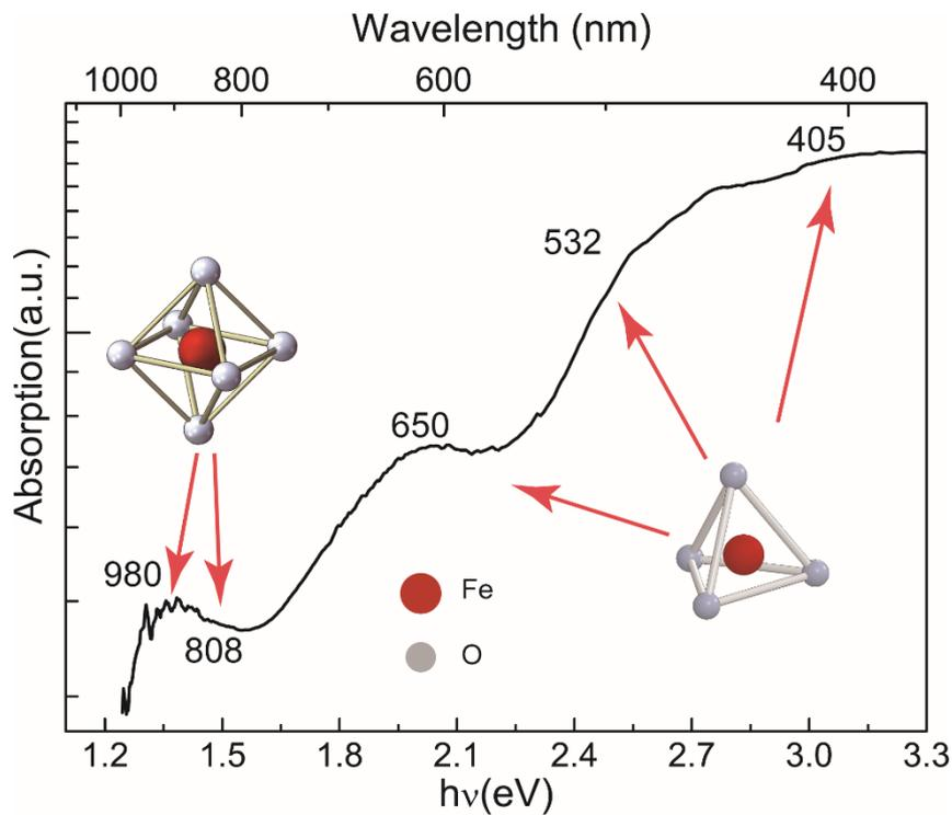
**Figure 4 | Absorption spectrum of YIG prepared by PLD.**
