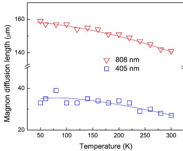
**Figure 3 | Temperature dependence of thermal magnon diffusion length.** The laser power is fixed at 30 mW. The solid lines are guides to the eyes.
