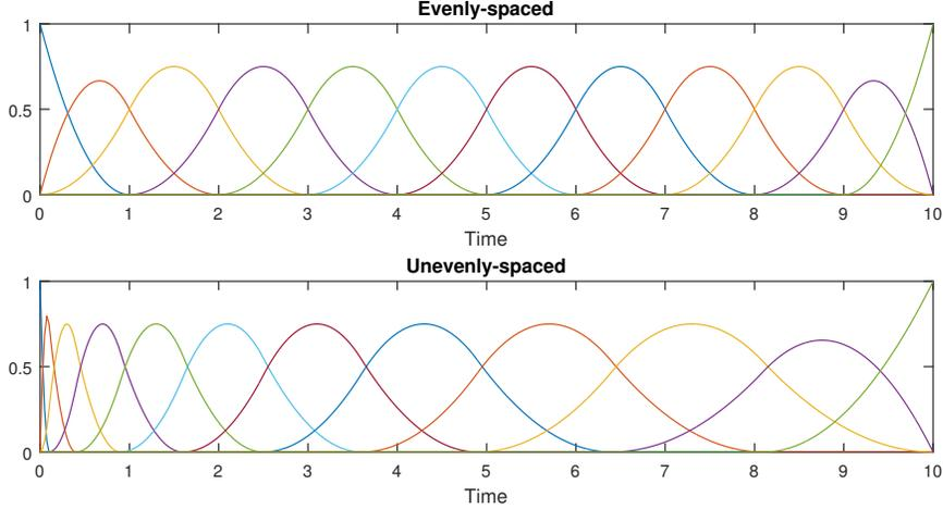
Figure 4: Upper plot: A set of 12 evenly-spaced B-splines in the interval  $[0, 10]$ . Lower plot: A set of 12 unevenly-spaced B-splines in the interval  $[0, 10]$  where more resolution is put on the early times.
