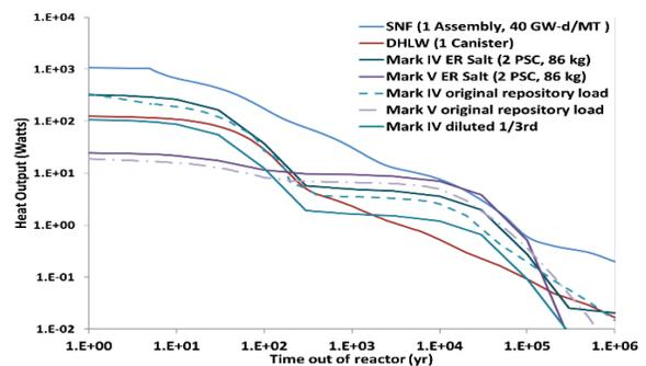
Fig. 2. Heat output from ER salt waste compared to a HLW canister and an SNF assembly.
