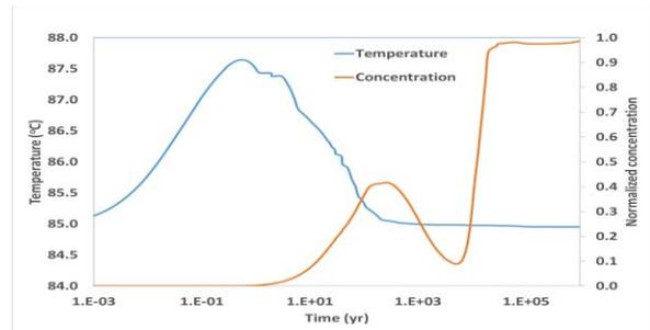
**Fig. 3. Temperature and salt concentration as function of time in borehole at 3000-m depth.**
