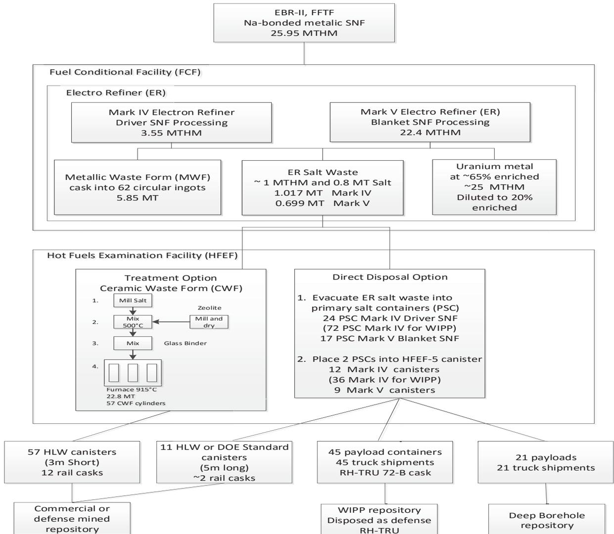
**Fig. 1. Various Pathways for Disposal of Na-Bonded SNF from EBR-II and FFTF.**
