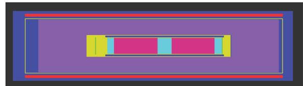
**Fig. 6. RH-TRU 72-B cask with dunnage (purple region) and additional shielding when transporting one HFEF-5**
