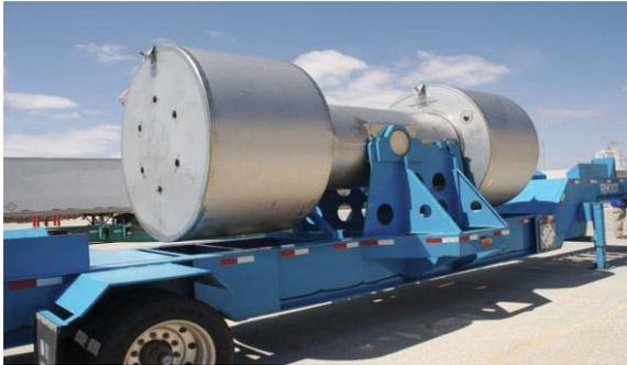
**Fig. 5. RH-TRU 72-B cask for remote-handled TRU.**
