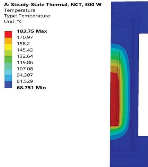
Fig. 7. Temperatures within RH-TRU 72-B with 2 PSCs at 300 W inside a standard payload canister as calculated by ANSYS (Rev 17.1) for normal transport conditions.
