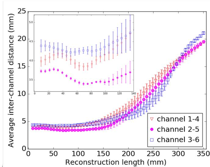
Figure 3 – Computed inter-channel distance along the reconstruction path. The insert correspond to the shielded-only portion. The dashed line are the geometrical error tolerance. The nominal inter-channel distance is 4 mm.
