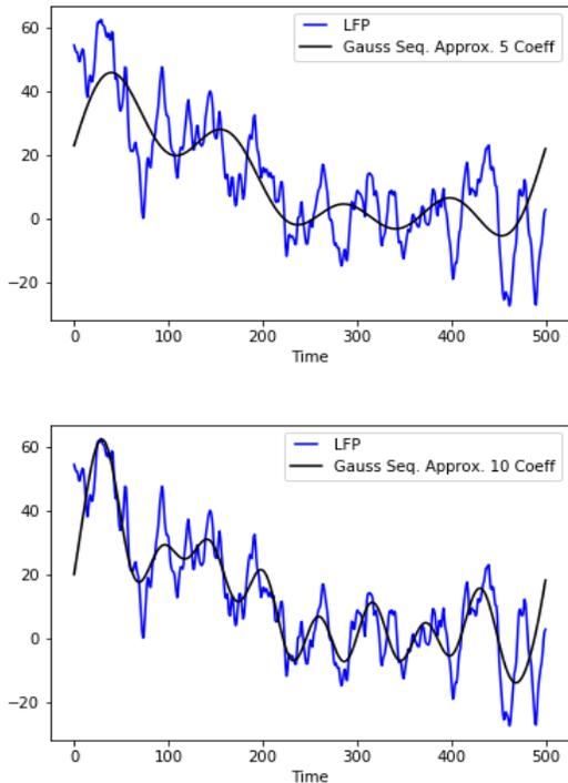
**Fig. 3:** Sample LFP waveform and its reconstruction using first 5 and 10 Fourier coefficients. Estimation is better with 10 coefficients, but classification performance was better with 5 coefficients.
