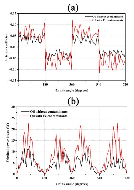
**Figure 3.** Tribological behavior versus crank angle with and without contaminants using  $1.1 \text{ m s}^{-1}$  average sliding speed, contaminants grain size of 20 µm, contaminants concentration of 40 ppm
