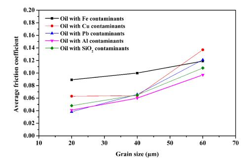
**Figure 5.** Effect of contaminants grain size on boundary friction coefficient using contaminants concentration of 60 ppm, 0.63 m s<sup>-1</sup> average sliding speed and 120 N normal load.
