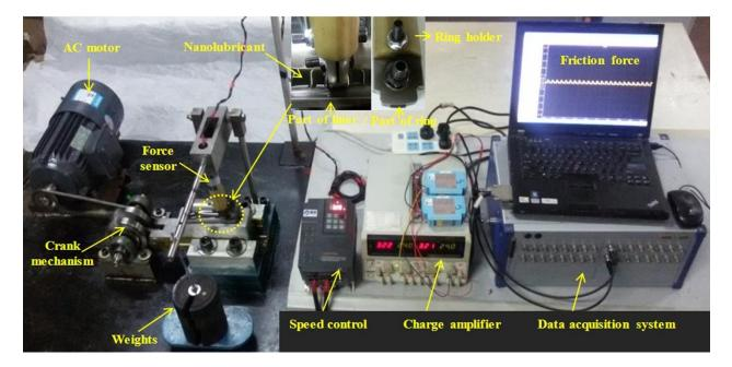
Figure 2. The test rig of the piston ring/cylinder liner interface designed.
