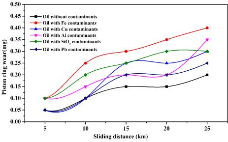
Figure 7. Comparisons of piston ring wear for different contaminants using concentration of 100
