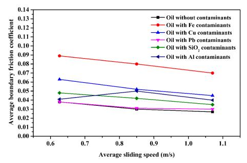
Figure 6. Effect of reciprocating sliding speed on average friction coefficient with different
