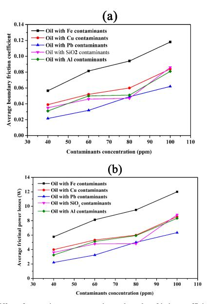
Figure 4. Effect of contaminants concentration on boundary friction coefficient (a) and power losses (b) under contaminants grain size of  $20 \ \mu m$ ,  $0.85 \ m s^{-1}$  average sliding speed and  $120 \ m m$  normal load.
