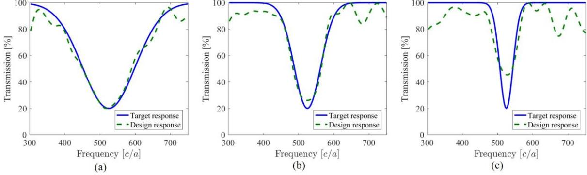
FIG. 6. Example design by the tandem neural network. The blue lines are Gaussian shaped target spectra, and the green lines are spectra of tandem network designs.
