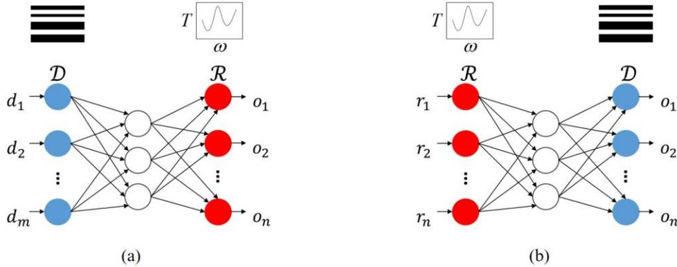
FIG. 1. (a) A forward modeling neural network with one hidden layer. The neural network takes device designs  $\mathcal{D}$  as inputs and outputs corresponding responses  $\mathcal{R}$ . (b) An inverse network with one hidden layer. It takes device responses  $\mathcal{R}$  as the input and outputs the designs  $\mathcal{D}$ .
