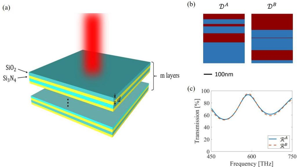
FIG. 2. (a) A thin film composed of  $m$  layers of  $\text{SiO}_2$  and  $\text{Si}_3\text{N}_4$ . The design parameters of the thin film are the thicknesses of the layers  $d_i$  ( $i=1, 2, \dots, m$ ) and the device response is the transmission spectrum. The forward neural network takes  $\mathcal{D}=[d_1, d_2, \dots, d_m]$  as inputs and discretized transmission spectrum  $\mathcal{R}$  as output. (b)(c) Example of two 6-layer thin film designs with very similar transmission spectra.
