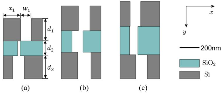
FIG.7. Designed structures of cases (a) (b) and (c) in Table 1.
