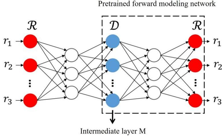
FIG. 4. A tandem network is composed of an inverse design network connected to a forward modeling network. The forward modeling network is trained in advance. In the training process, weights in the pre-trained forward modeling network are fixed and the weights in the inverse network are adjusted to reduce the cost (i.e., error between the predicted response and the target response). Outputs by the intermediate layer M (labeled in blue) are designs  $\mathcal{D}$ .
