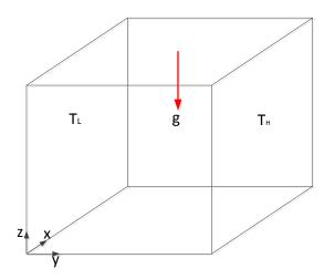
Figure 1: Geometric configuration for the physical model of the 3D cubic cavity and the coordinate system.
