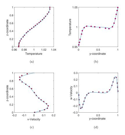
Figure 2: Comparison of the temperature (top) and velocity profiles (bottom) for Rayleigh number Ra =  $10^5$  on the symmetry (x = 0.5) center plane y - z; symbols " $\circ$ " denote the reference benchmark solutions [33], and lines "-" represent results obtained using 3D thermal cascaded LBM.
