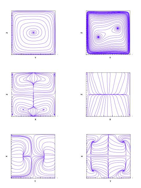
Figure 3: Projections of streamlines in natural convection in a 3D cavity computed using 3D thermal cascaded LBM along different center planes at Rayleigh numbers  $Ra = 10^4$  (left) and  $Ra = 10^5$  (right). Top row: y - z plane, Middle row x - z plane, Bottom row: y - x plane.
