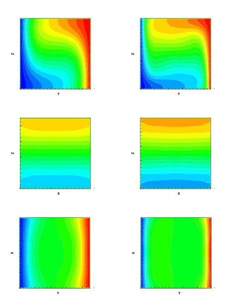
Figure 4: Temperature distribution in natural convection in a 3D cavity computed using 3D thermal cascaded LBM along different center planes at Rayleigh numbers  $Ra = 10^4$  (left) and  $Ra = 10^5$  (right). Top row: y - z plane, Middle row x - z plane Bottom row: y - x plane.
