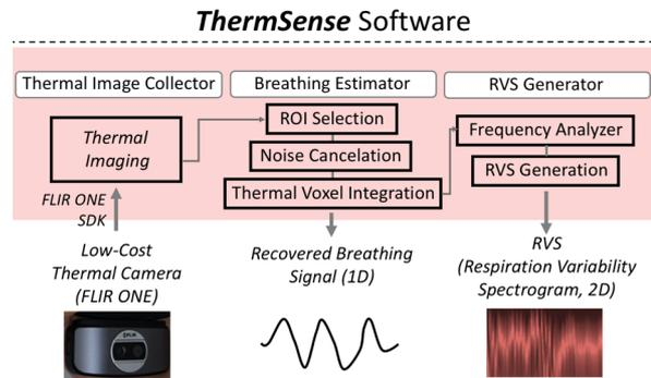
Figure 1. Software architecture of ThermSense: it consists of three parts – continuous thermal image extractor, breathing estimator and respiration variability spectrogram (RVS) generator.
