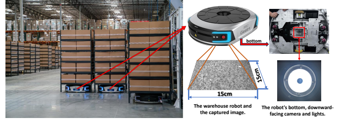
Fig. 1. In the warehouse, dynamic objects (robots and storage racks) and large-scale environments make the localization with a forward-facing camera or LiDAR very challenging, so currently, a downward-facing camera is usually used to detect tags deployed on the ground for stable localization. To eliminate this limitation, we developed a non-iterative SLAM for warehouse robots. It provides robust localization with 78% improvements over the state-of-the-art (SOTA) SLAM systems on various ground textures.
